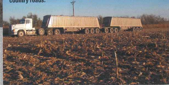
A tandem trailer rig awaiting its load in a South Dakota field illustrates the challenge rural road managers face today. Big rigs like this, a common sight on rural roads today as they haul material from field to farm and from farm to market, dramatically increase the load capacity requirements for country roads.
