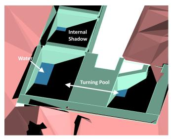
Figure 8: View of turning pool of fish ladder and internal shadows, on June 21st at 7:00 AM (looking west along the southern river bank from a bird's eye perspective)
