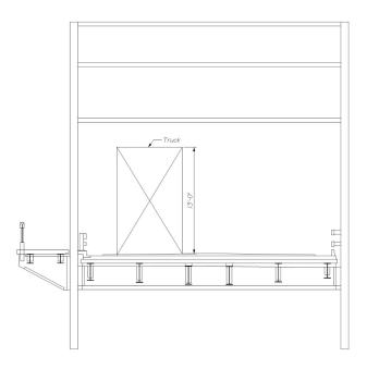
Figure 5: Existing Truss Bridge Modeled Cross Section
