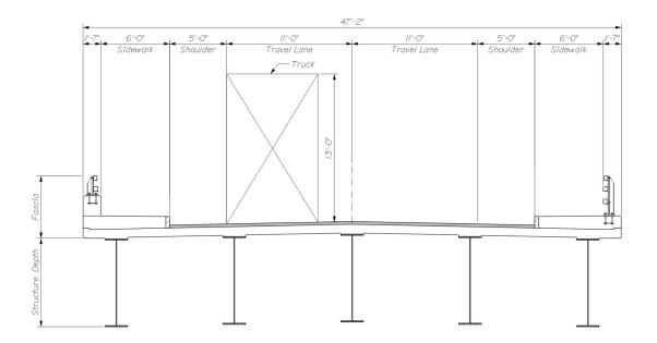
Figure 6: Proposed Upstream Curved Bridge Modeled Cross Section
