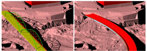
Figure 3: 3D Models of Existing Truss and Proposed Curved Bridges
