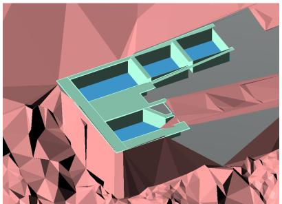
Figure 4: 3D model of fish ladder turning pool and adjacent pools
