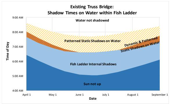
Figure 10: Existing Truss Bridge Shadow Times
