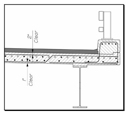
Figure 8-1 Cover Requirements in Superstructure
