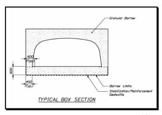
Figure 5-14 Structural Plate Box Culvert Typical Section
