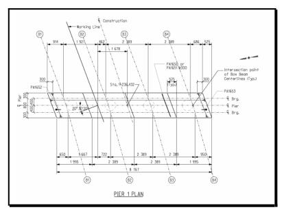
Figure 3-25 Pile Bent Pier Plan
