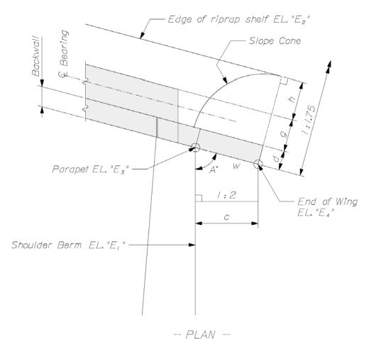
(Stub or integral abutment with riprap shelf)
