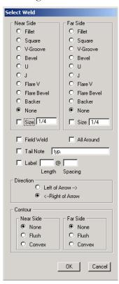
Figure 9-4 MicroStation Weld Symbol Macro
