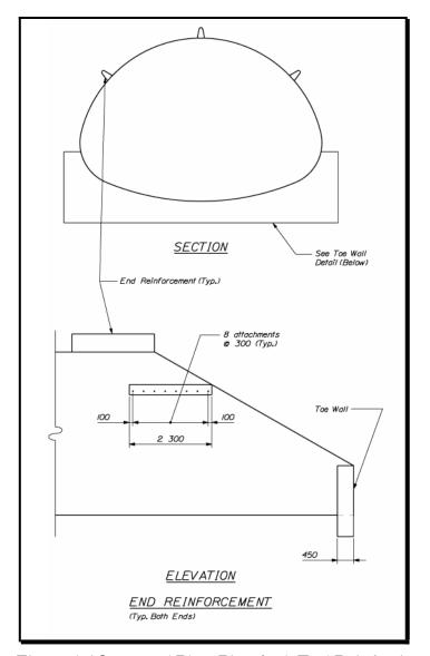
Figure 5-6 Structural Plate Pipe Arch End Reinforcing
