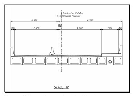
Figure 7-13 Staged Construction (Final Stage)
