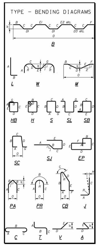
Figure 8-21 Bent Types
