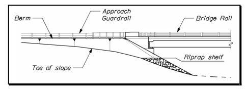
Figure 3-9 Return Wing Elevation
