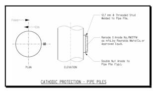
Figure 3-29 Pile Bent Pier Cathodic Protection - Pipe Piles
