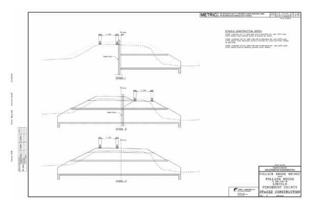
Figure 7-9 Staged Construction Sheet (Buried Structure)
