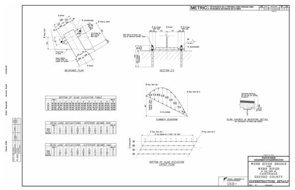
Figure 4-3 Steel Girder Superstructure Details
