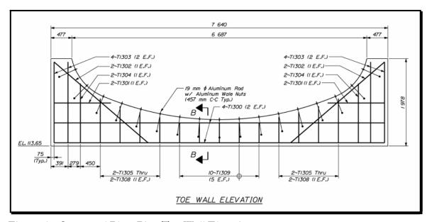
Figure 5-7 Structural Plate Pipe Toe Wall Elevation
