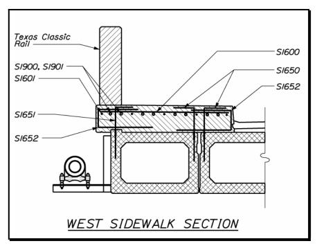
Figure 7-33 Utility on Exterior Box Beam
