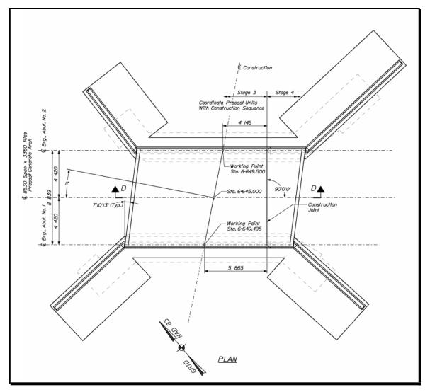
Figure 5-24 Precast Concrete Arch Plan
