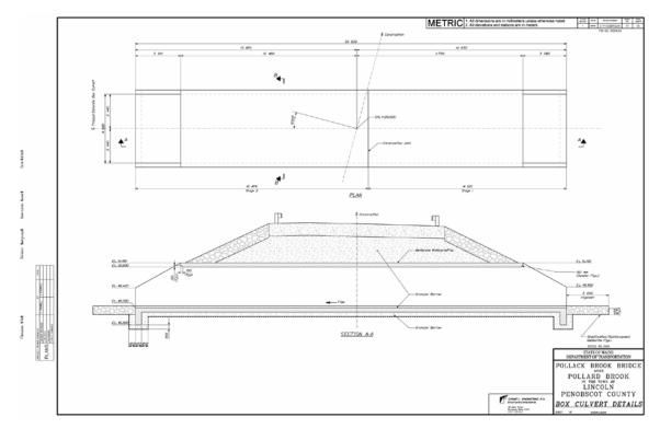
Figure 5-17 Box Culvert Details
