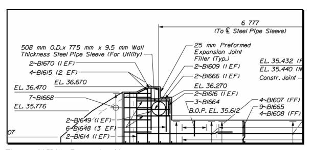
Figure 7-34 Utility Penetrating Abutment
