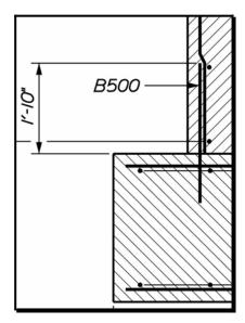
Figure 8-7 Dowel Projection
