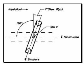
Figure 2-6 Layout of Culvert
