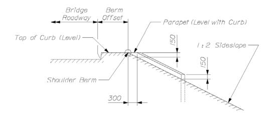
(Elevation at Back of Abutment)
