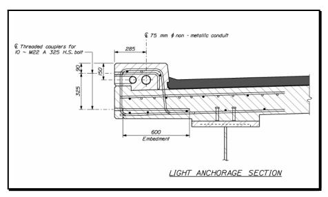
Figure 7-29 Light Anchorage Section
