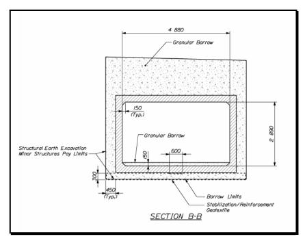
Figure 5-20 Precast Concrete Box Culvert Typical Section
