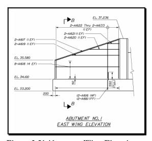
Figure 3-21 Abutment Wing Elevation
