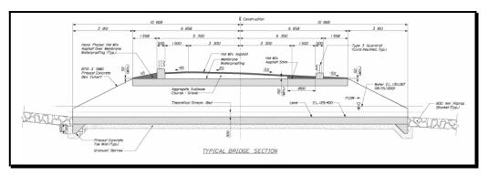
Figure 2-13 Proposed Bridge Section (Buried Structures)
