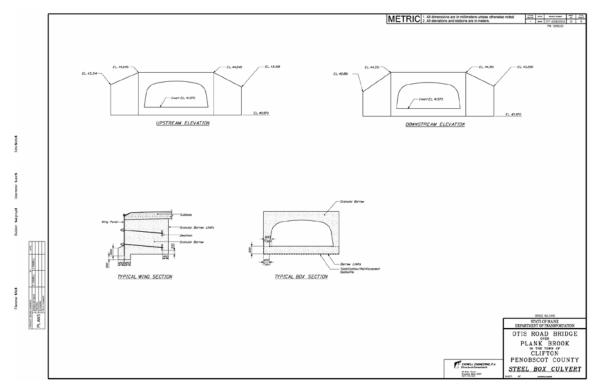
Figure 5-11 Steel Box Culvert Details Sheet
