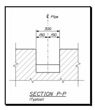
Figure 7-25 Transverse Notch Section
