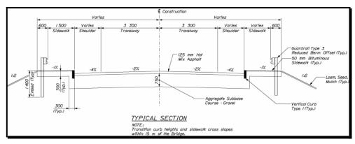
Figure 2-25 Approach Design Section
