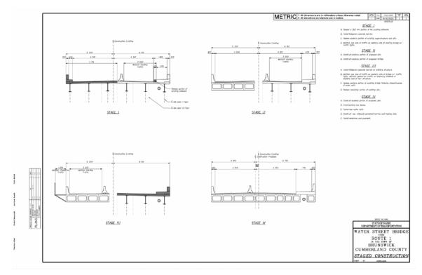
Figure 7-8 Staged Construction Sheet (Typical Bridge)
