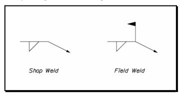
Figure 9-7 Shop Weld vs. Field Weld
