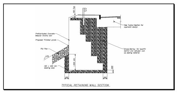
Figure 3-36 Wall Section
