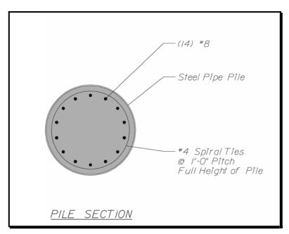
Figure 3-28 Pile Bent Pier Typical Pile Section
