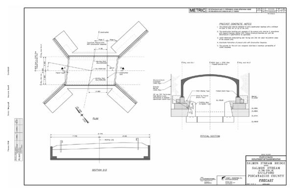
Figure 5-21 Arch / Rigid Frame Details
