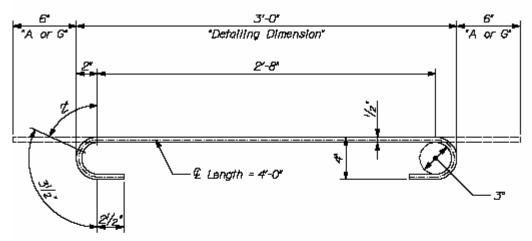
~ BAR DIMENSIONS PER "CRSI STANDARD HOOK DETAILS" ~ (Example bar size #4 shown)
