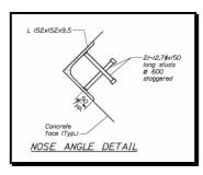
Figure 3-33 Solid Pier Nose Angle Detail
