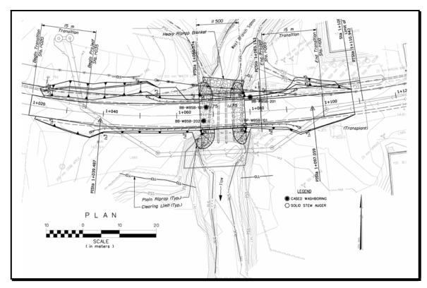
Figure 7-5 Boring Location Plan
