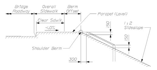
(Elevation at Back of Abutment)
