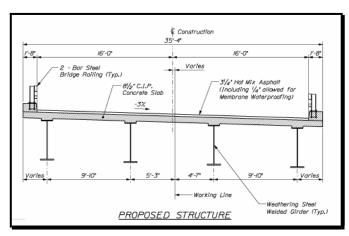
Figure 2-12 Proposed Bridge Section (Traditional Bridge)
