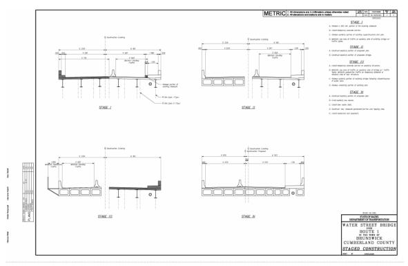
Figure 2-10 Preliminary Staged Construction Sheet
