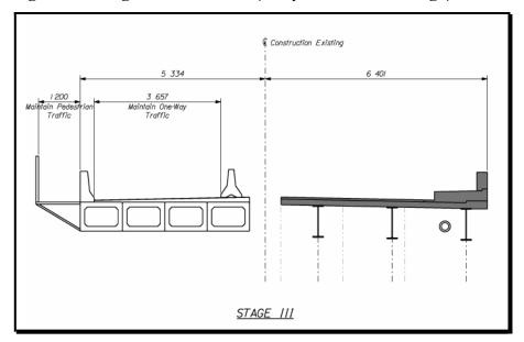
Figure 7-12 Staged Construction (Late Intermediate Stage)
