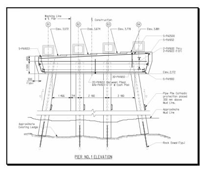
Figure 3-26 Pile Bent Pier Elevation
