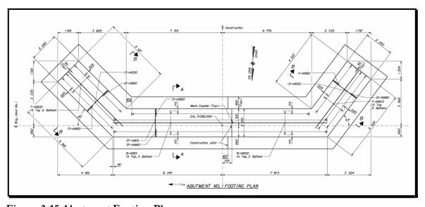
Figure 3-15 Abutment Footing Plan
