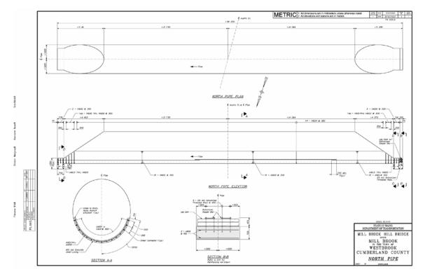
Figure 6-1 Invert Lining Sheet
