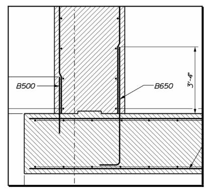
Figure 8-3 Unenclosed Hook
