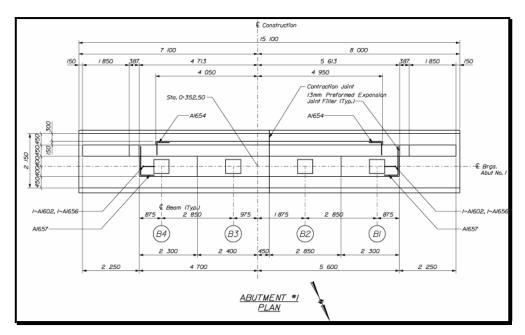
Figure 3-17 Abutment Plan
