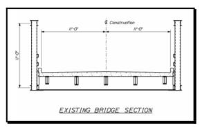
Figure 2-11 Existing Bridge Section
