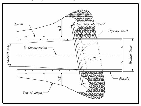
Figure 3-6 Extension Wing Plan
