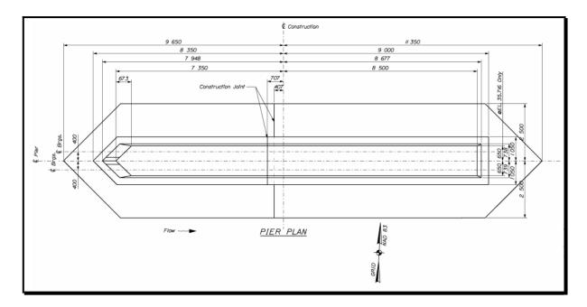
Figure 3-30 Solid Pier Plan
