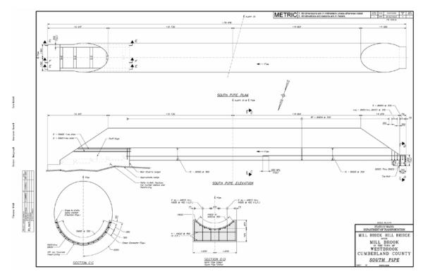
Figure 7-16 Structure Sheet with Fish Weir
