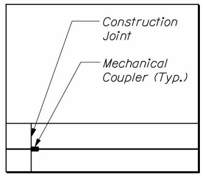
Figure 8-6 Mechanical Coupler
