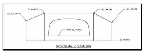
Figure 5-15 Structural Plate Box Culvert Headwall and Wing Elevation
