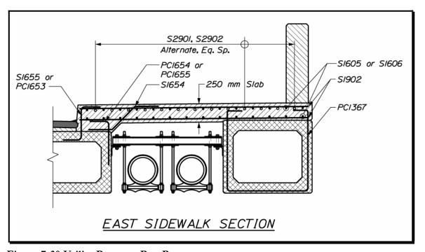
Figure 7-30 Utility Between Box Beams
