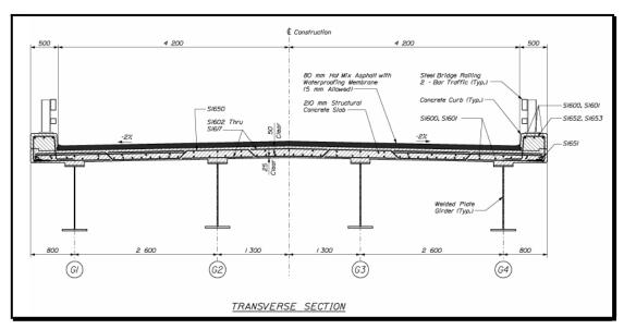
Figure 4-6 Steel Girder Transverse Section
