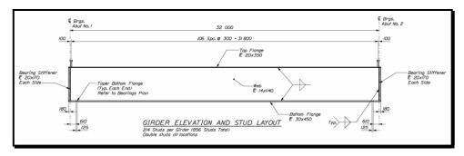
Figure 9-8 Welded Plate Girder Weld Example
