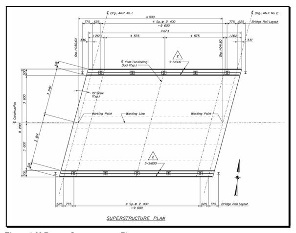
Figure 4-22 Precast Superstructure Plan
