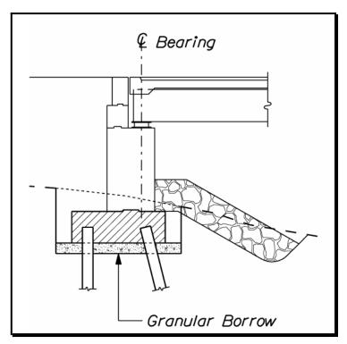
Figure 3-4 Footing On Piles
