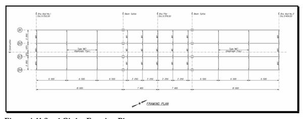
Figure 4-11 Steel Girder Framing Plan
