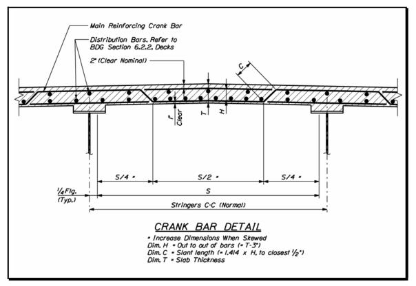
Figure 8-18 Crank Bar Detail
