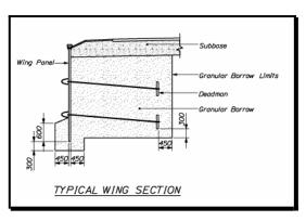
Figure 5-16 Structural Plate Box Culvert Typical Wing Section
