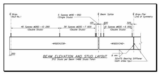
Figure 4-12 Steel Girder Beam Elevation and Stud Layout
