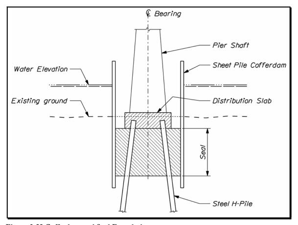
Figure 3-22 Cofferdam and Seal Foundation
