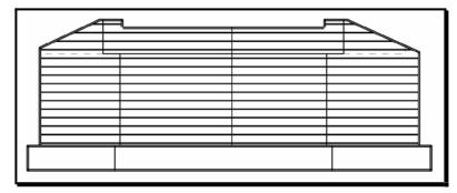
Figure 8-16 Working Sketch of Abutment Elevation
