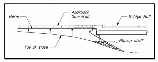
Figure 3-11 Flared Wing Elevation
