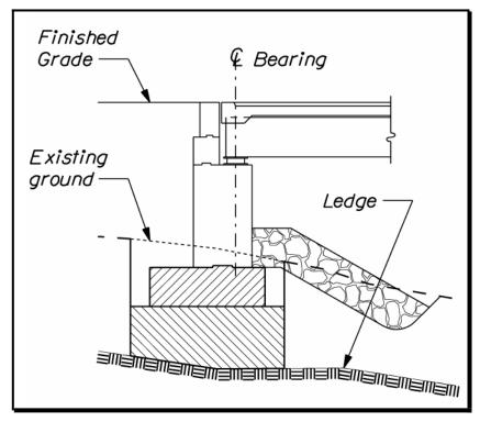
Figure 3-3 Footing On Concrete Fill
