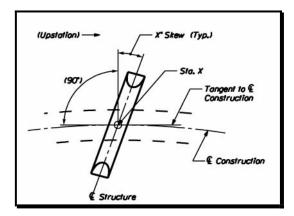
Figure 2-7 Layout of Culvert on Curve
