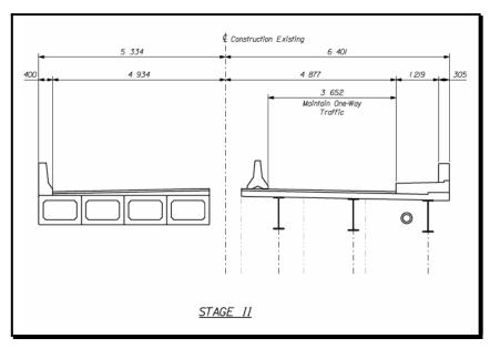
Figure 7-11 Staged Construction (Early Intermediate Stage)
