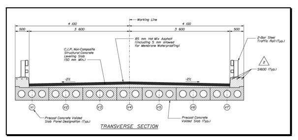
Figure 4-23 Precast Transverse Section
