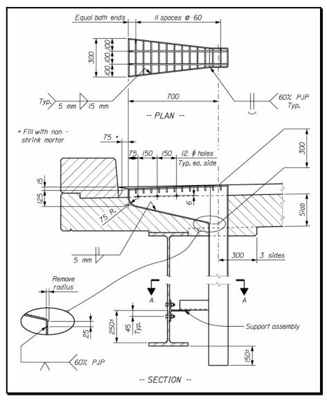
Figure 9-9 Bridge Drain Weld Example
