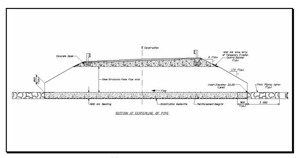
Figure 5-4 Structural Plate Pipe Transverse Section
