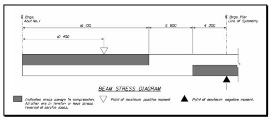
Figure 4-14 Steel Girder Beam Stress Type Diagram
