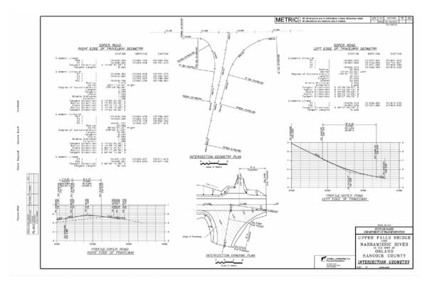
Figure 2-18 Intersection Layout Sheet
