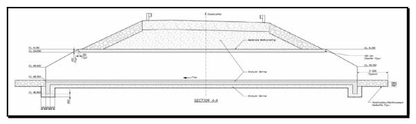
Figure 5-19 Precast Concrete Box Culvert Longitudinal Section
