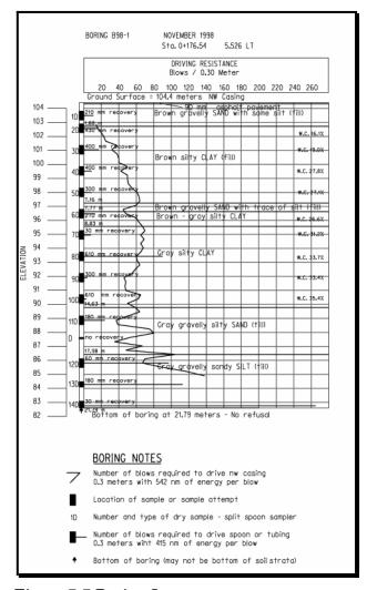
Figure 7-7 Boring Logs
