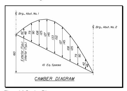
Figure 4-8 Camber Diagram
