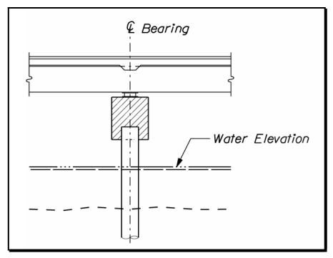
Figure 3-23 Pile Bent Foundation
