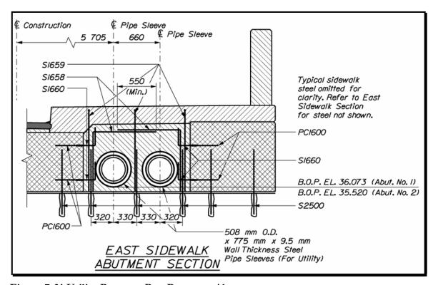
Figure 7-31 Utility Between Box Beams at Abutment
