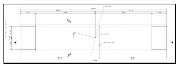
Figure 5-18 Precast Concrete Box Culvert Plan
