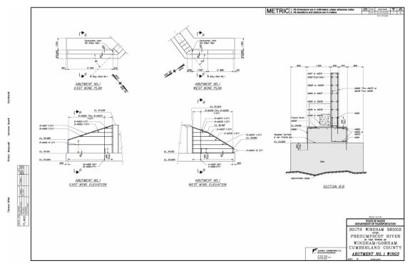
Figure 3-14 Abutment Wings Sheet
