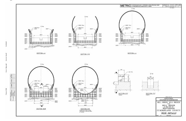
Figure 7-18 Weir Details Sheet 2
