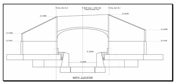
Figure 5-27 Precast Concrete Arch End Elevation
