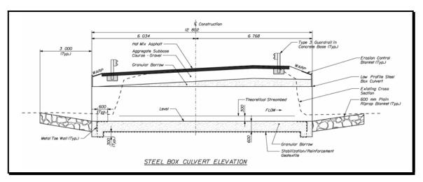
Figure 5-13 Structural Plate Box Culvert Longitudinal Section
