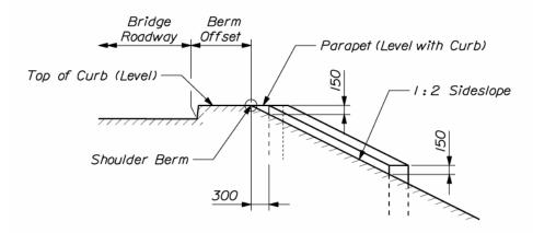
(Elevation at Back of Abutment)
