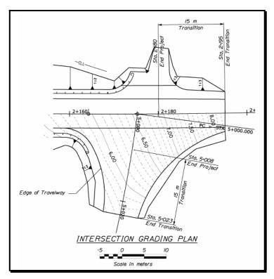
Figure 2-23 Intersection Grading Plan
