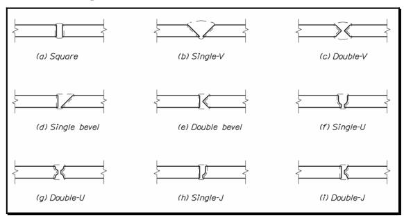
Figure 9-3 Types of Groove Welds
