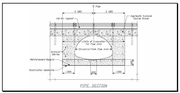
Figure 5-5 Structural Plate Pipe Arch Typical Section
