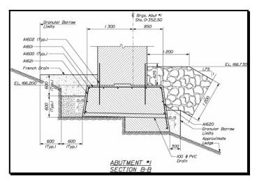
Figure 3-16 Abutment Footing Section
