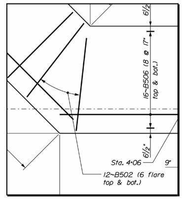
Figure 8-20 Flare Bars in Footing
