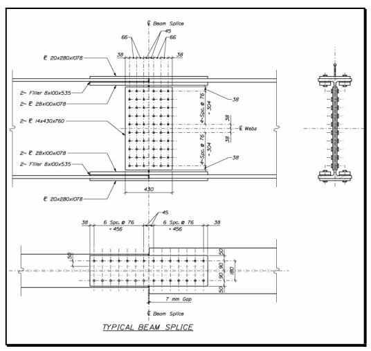
Figure 4-13 Steel Girder Field Splice Details
