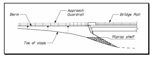
Figure 3-7 Extension Wing Elevation
