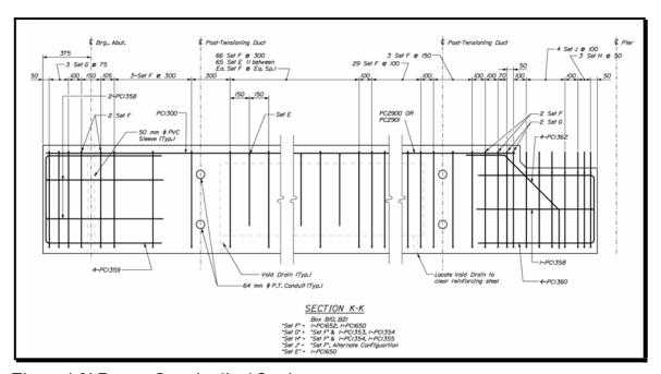
Figure 4-21 Precast Longitudinal Section
