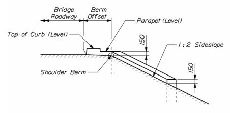
(Elevation at Back of Abutment)
