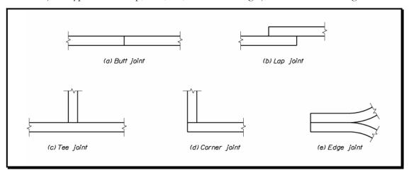
Figure 9-1 Common Types of Welded Joints
