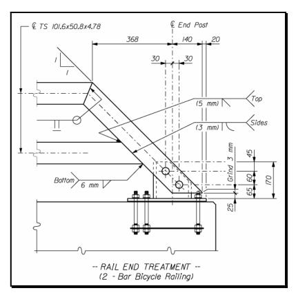
Figure 9-10 Rail End Treatment Weld Example
