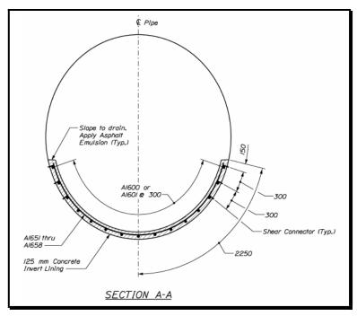
Figure 6-4 Invert Lining Section
