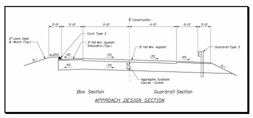
Figure 2-14 Approach Design Section
