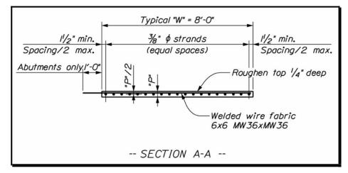
Figure 8-19 Welded Wire Fabric
