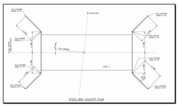
Figure 5-12 Structural Plate Box Culvert Plan
