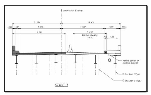
Figure 7-10 Staged Construction (Stage I)
