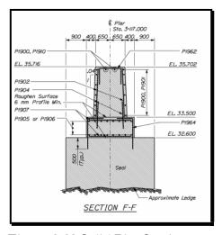
Figure 3-32 Solid Pier Section
