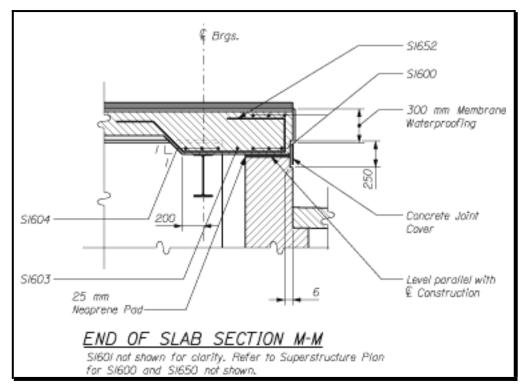
Figure 4-7 Steel Girder End of Slab Section
