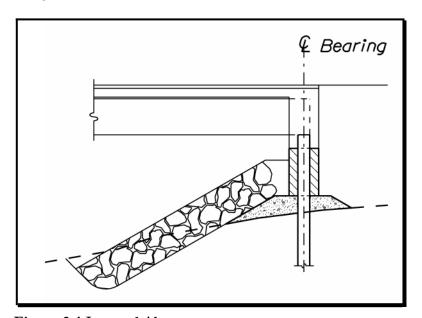
Figure 3-1 Integral Abutment
