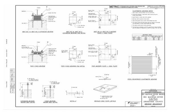
Figure 4-4 Steel Girder Bridge Bearings Sheet
