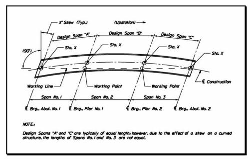
Figure 2-4 Layout of Bridge on a Curve
