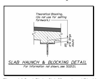
Figure 4-9 Steel Girder Slab Haunch and Blocking Detail
