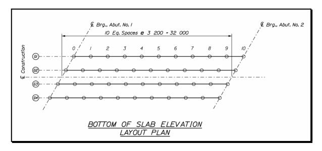
Figure 4-10 Steel Girder Bottom of Slab Elevation Layout Plan
