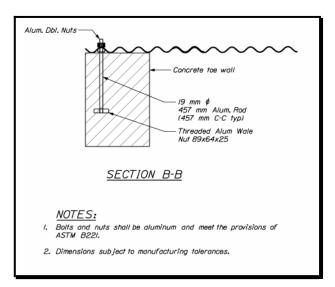
Figure 5-8 Structural Plate Pipe Toe Wall Section
