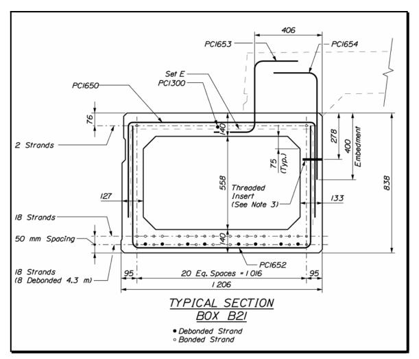
Figure 7-32 Threaded Inserts in Precast Concrete
