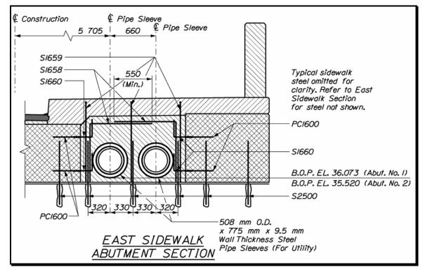
Figure 7-31 Utility Between Box Beams at Abutment
