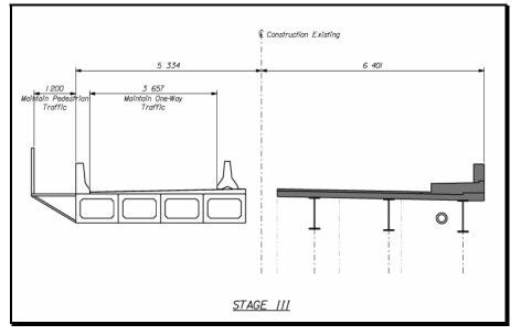
Figure 7-12 Staged Construction (Late Intermediate Stage)
