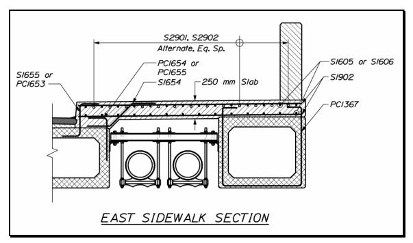
Figure 7-30 Utility Between Box Beams
