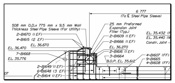
Figure 7-34 Utility Penetrating Abutment
