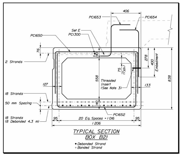
Figure 7-32 Threaded Inserts in Precast Concrete
