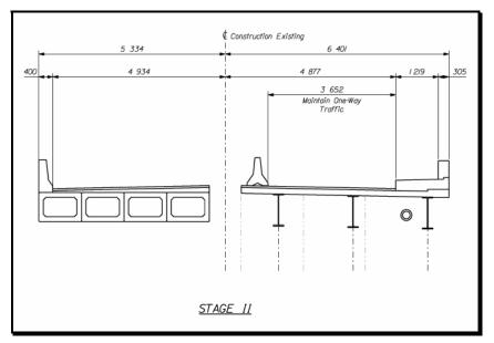
Figure 7-11 Staged Construction (Early Intermediate Stage)
