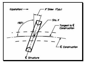
Figure 2-7 Layout of Culvert on Curve
