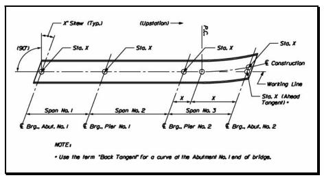
Figure 2-5 Layout of Bridge on a Partial Curve
