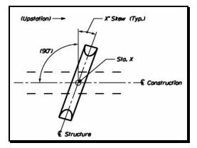
Figure 2-6 Layout of Culvert
