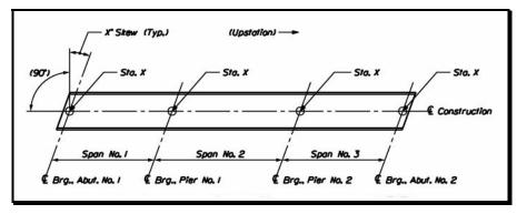
Figure 2-3 Layout of Bridge on a Tangent
