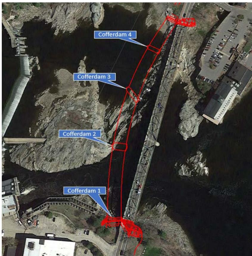
Figure 2-3. Schematic showing proposed locations of cofferdams required for installation of new Brunswick-Topsham Bridge.
