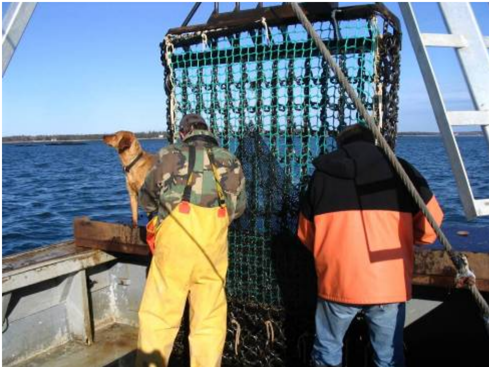
Photo 2. Sea urchin drag being configured with small mesh covering the bottom two-thirds of the back of the drag, to simulate an escape panel in the top third.
