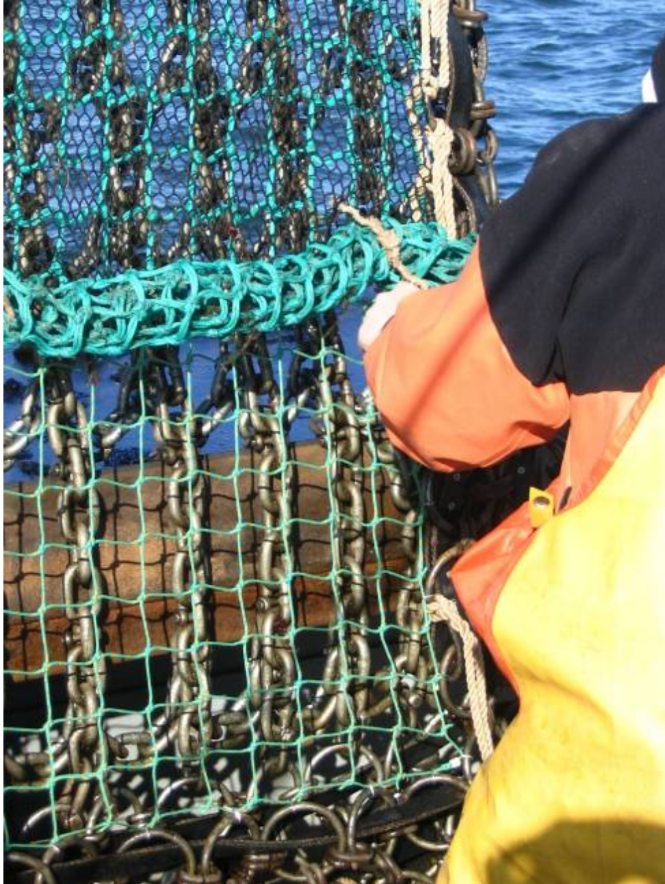
Photo 10. Reconfiguring the escape panel by rolling the 2-inch mesh out of the way and replacing with 2¼-inch mesh. Note smaller mesh covering the top two-thirds of the net, to simulate a 2¼-inch escape panel in the bottom third.
