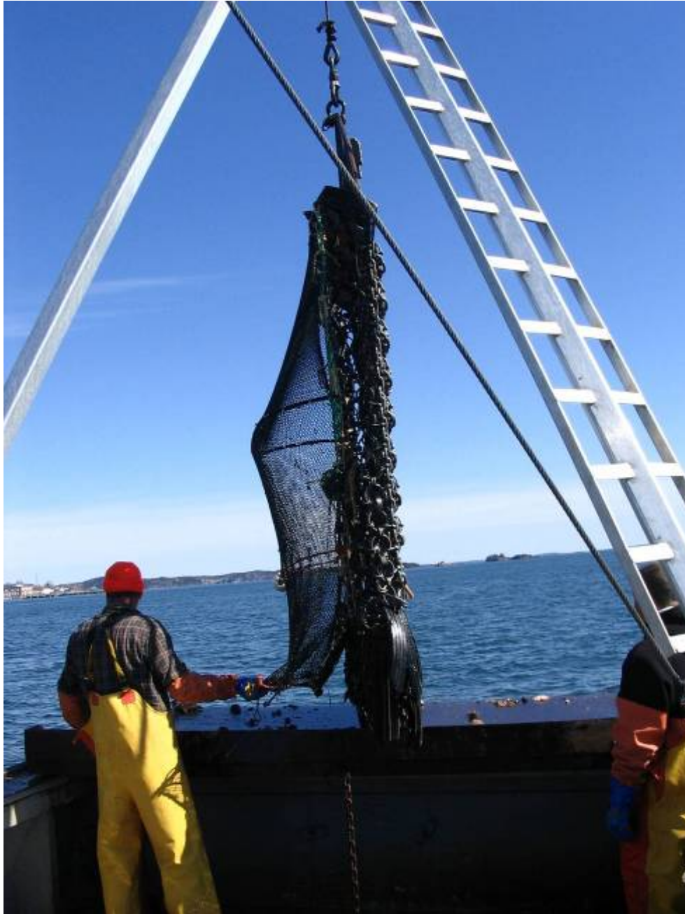
Photo 11. The outer bag catch purse on the back of the drag, designed to catch whatever escapes through the escape panel, which, in this case, is the bottom panel of the drag.
