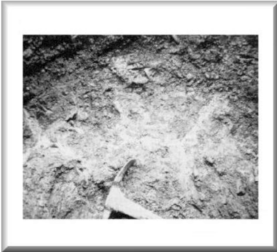
**Figure 53. Top view of prismatic structure in a subsoil**
