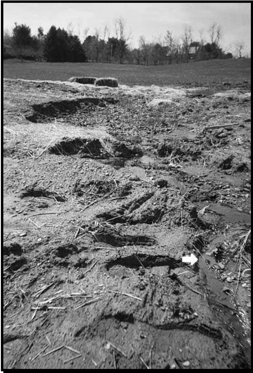
**Figure 66. Malfunction resulting in effluent breakout and overland runoff (arrow).**
