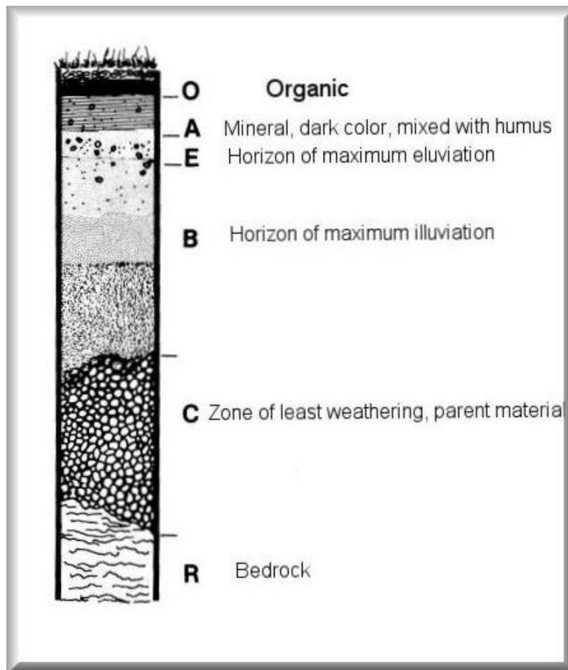
**Figure 39. Theoretical soil horization**
