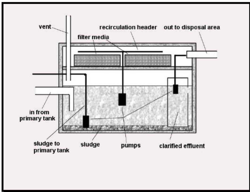
**Figure 30. Simplified cross section of a recirculating aerobic treatment tank.**
