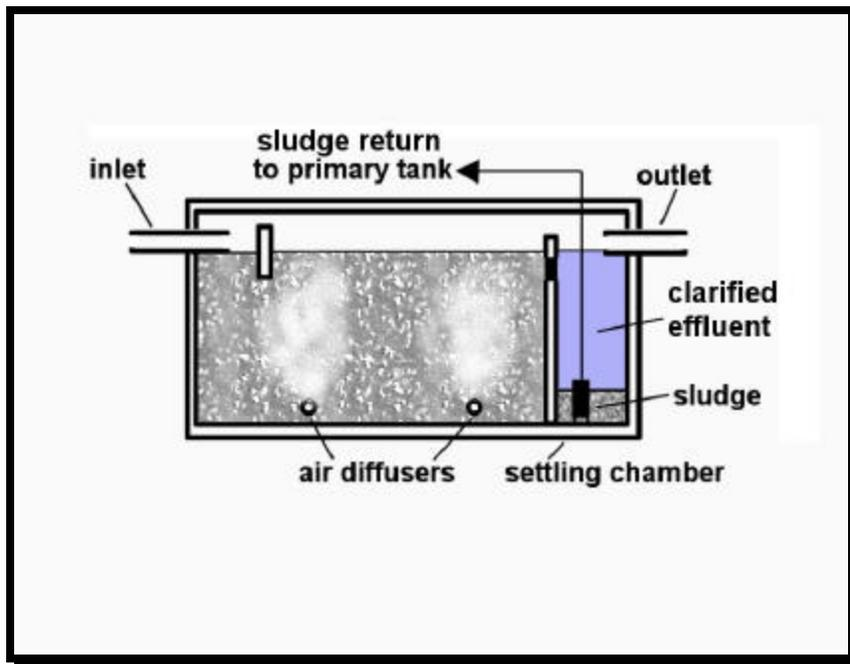
**Figure 28. Simplified cross section of an aerobic treatment unit.**
