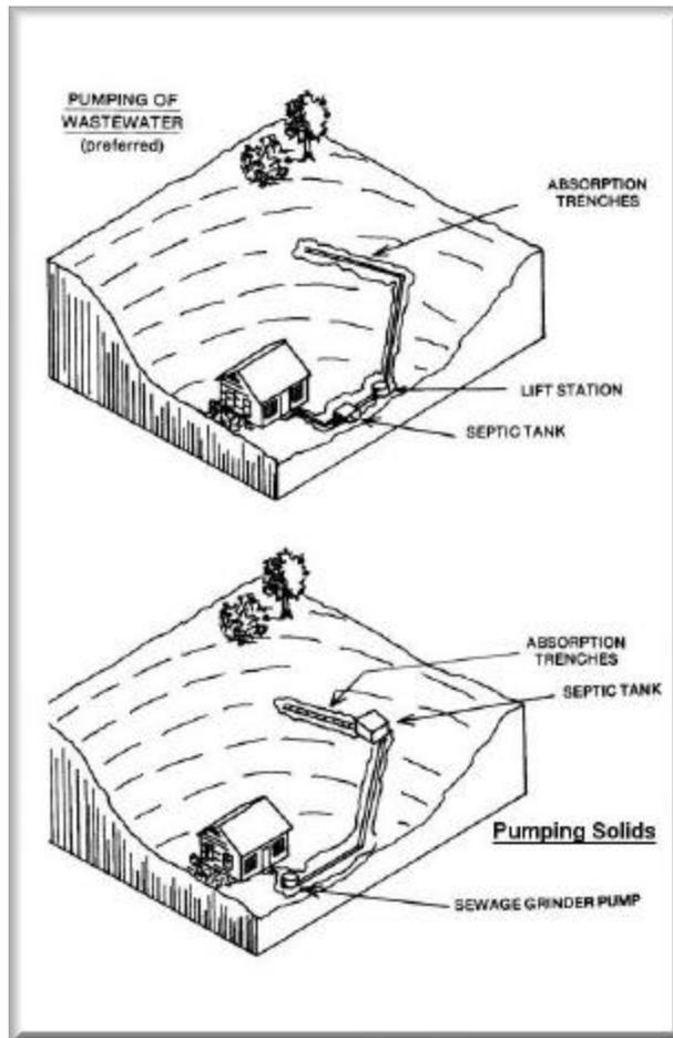
Figure 32. Effluent and sewage lift station design layouts
