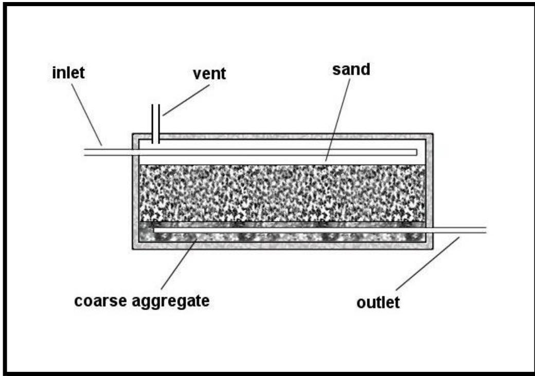
Figure 22. Cross section of under-drained sand filter.
