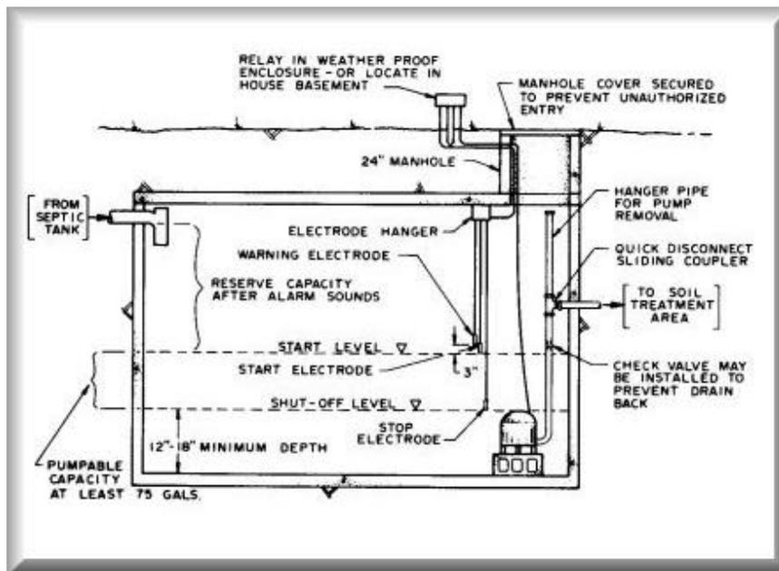
Figure 33. Pump tank and effluent pump for single family residence
