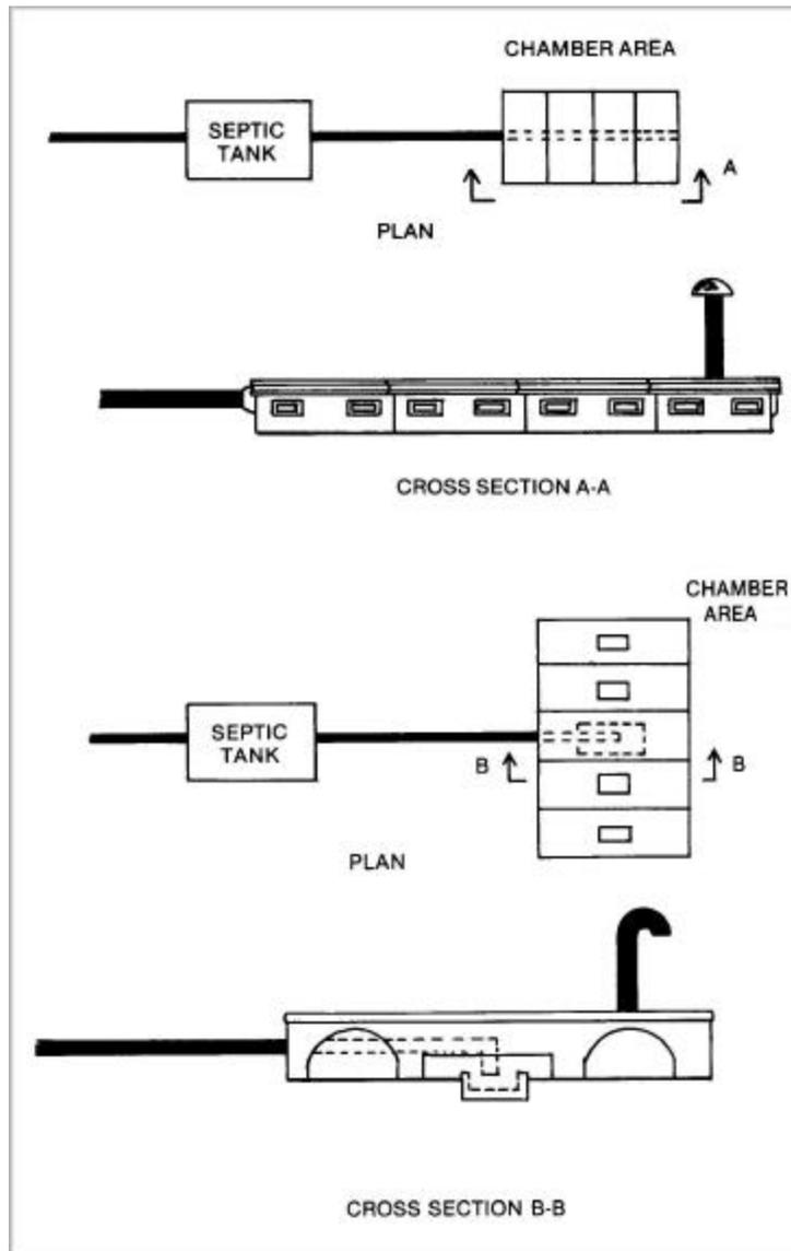
**Figure 10. Manufactured concrete chamber designs and distribution methods**
