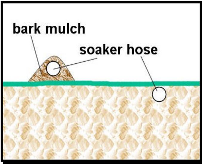
**Figure 19. Porous soaker hose drip irrigation system.**
