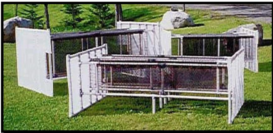
**Figure 27. Whole tank filters**
