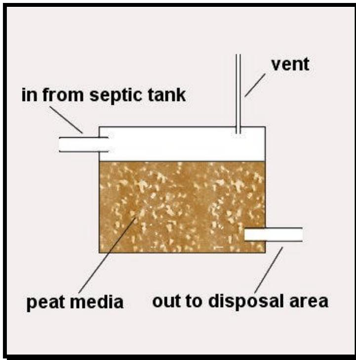
**Figure 21. Simplified cross section of a peat filter module.**
