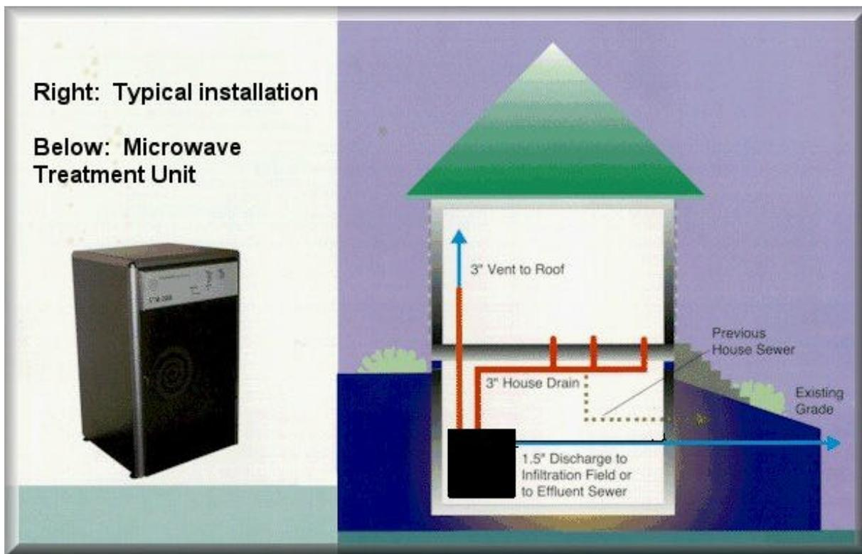
**Figure 31. Typical microwave residential installation.**
