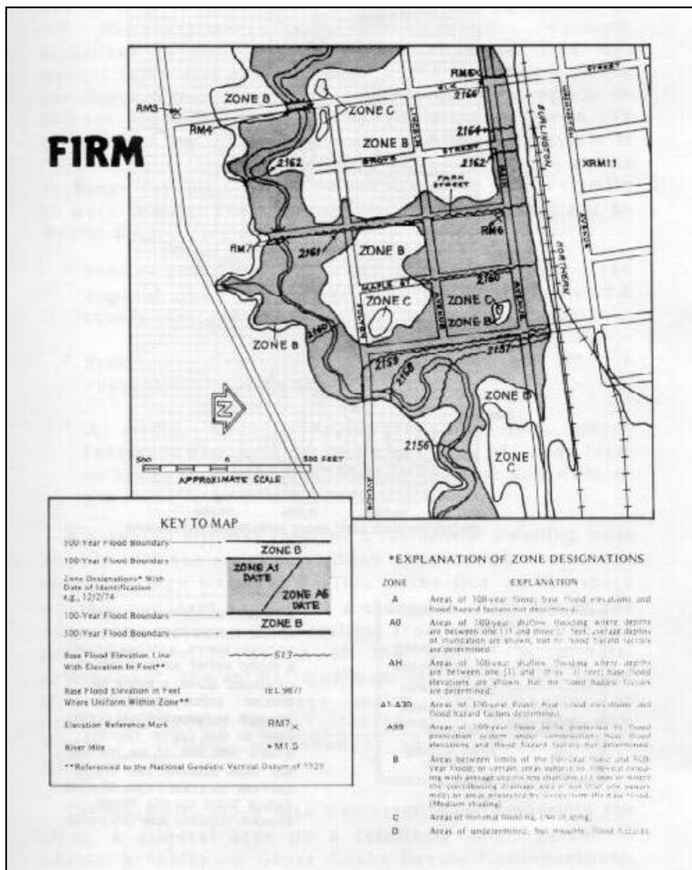
Figure 62. Flood Boundary, Floodway Map
