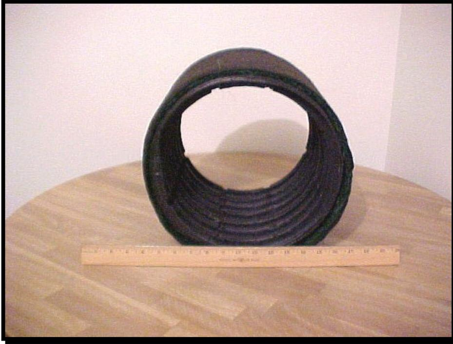
**Figure 14. Cross section of fabric covered tube.**
