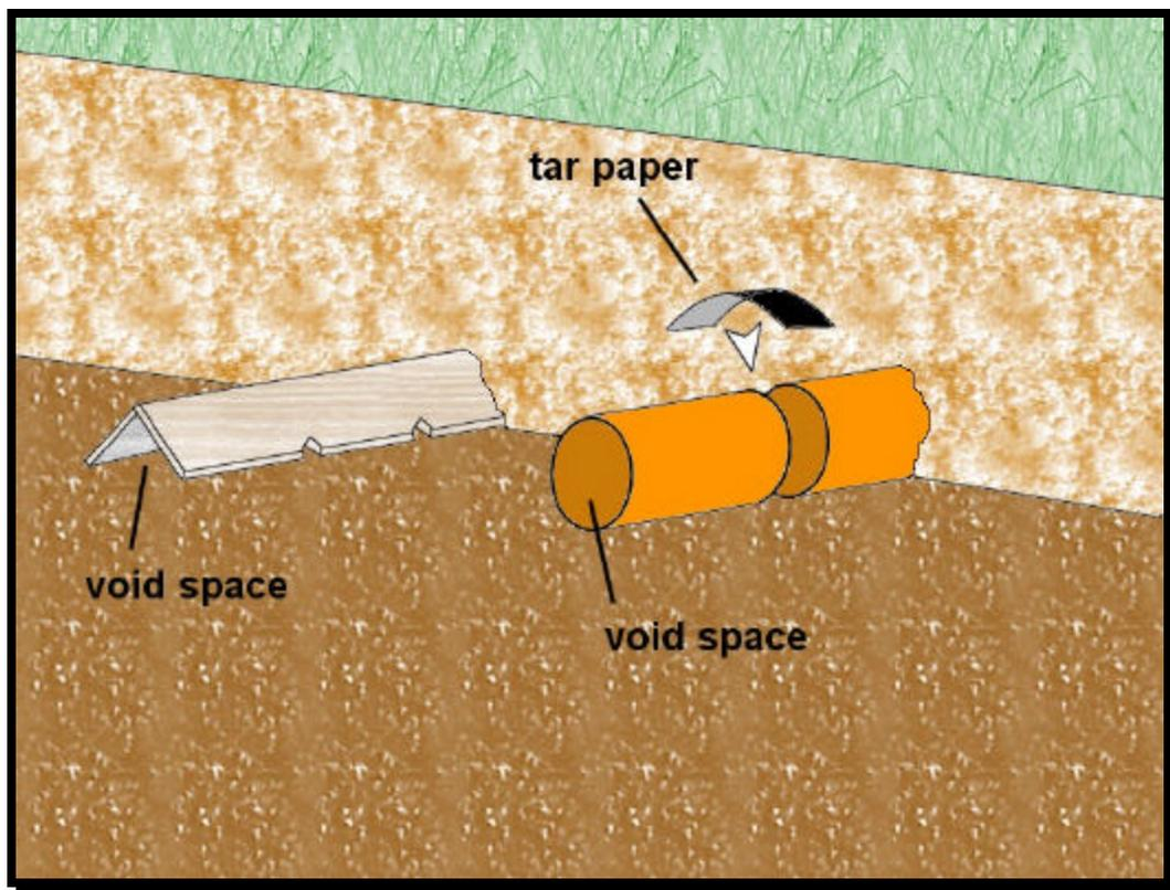
Fig 7. Comparison of Vee-Plank and Tile Trenches
