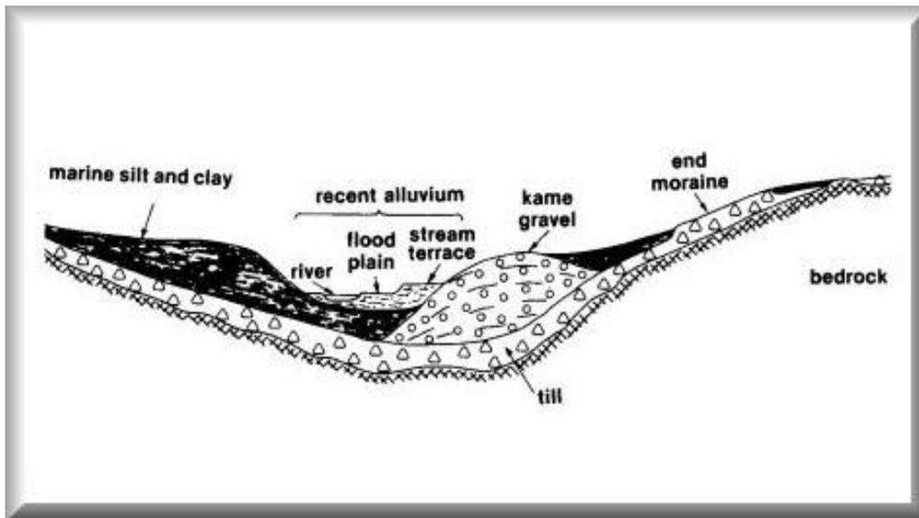
Figure 50. Cross section showing relationships among surficial deposits, generalized
