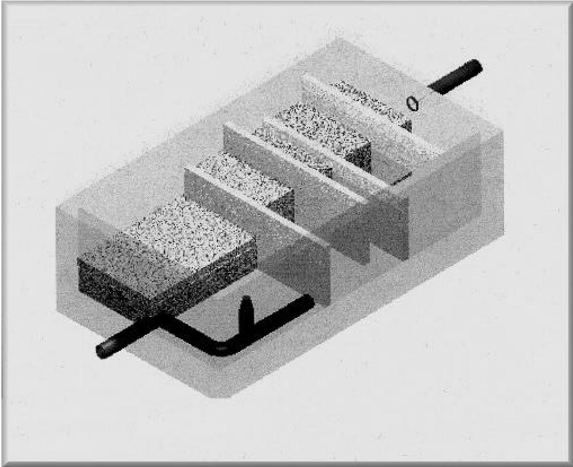
**Figure 23. Isometric cross section of graduated media filters.**
