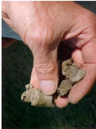
**Figure 42. Silty clay soil ribboning**
