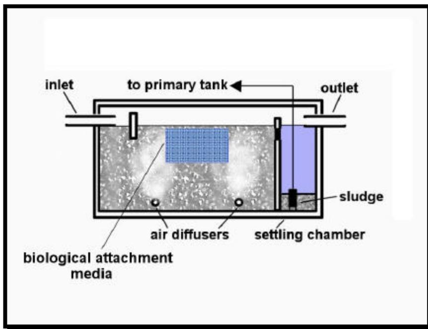
**Figure 29. Simplified cross section of a fixed film aerobic treatment unit.**
