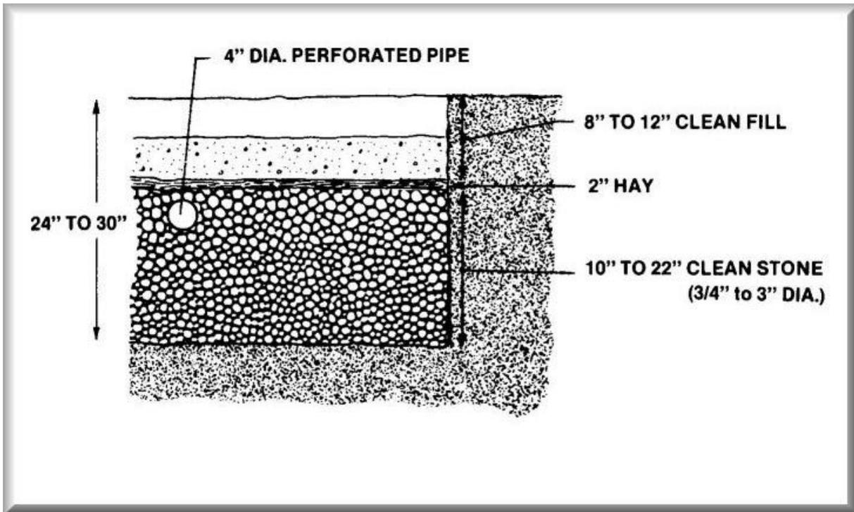
**Figure 4. Cross section of disposal bed**
