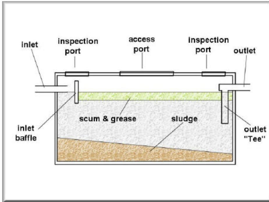
**Figure 2. Cross-section of a typical septic tank.**
