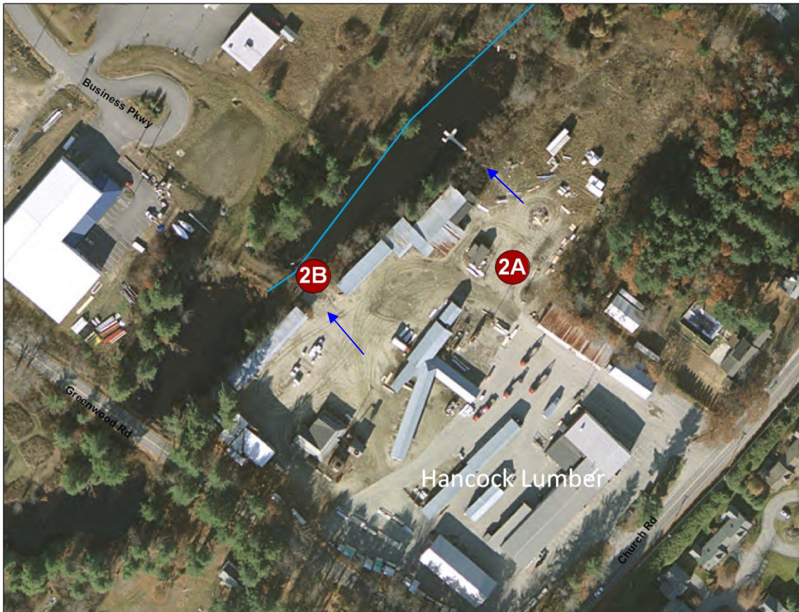
Figure 6: Location of potential stormwater mitigation Site 2 at Hancock Lumber off Church Rd. Blue arrows indicate direction of direct flow to stream.
