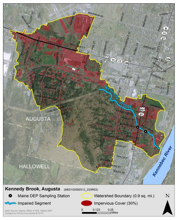
**Figure 1:** Map of Kennedv Brook watershed impervious cover.
