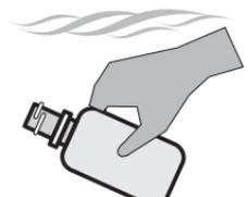
Remove the cap and allow the bottle to fill.
