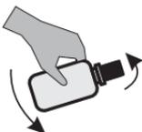
**NOTE:** At this point the sample has been "fixed" and contact between the sample and the atmosphere will not affect the test result. Samples may be held at this point and titrated later.
