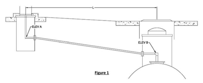
**Example:** A dispenser elbow (**ELEV A**) is surveyed at 6.280 ft. The tank top piping elbow (**ELEV B**) is surveyed at 5.238 ft. The piping length (**L**) is determined to be 86 ft. The elevation change (**E**) between the two elbows is 1.042 ft (or 12.5 inches), therefore the calculated slope (**S**) is 12.5 in  $\div$  86 ft = 0.145 in/ft. In this example, the calculated slope of 0.145 in/ft is more than the minimum of 0.125 in/ft and the piping has proper slope.
