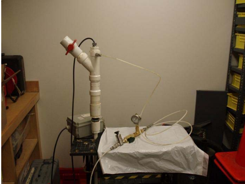
Figure 4. Pneumatic Slug Test Apparatus showing Well Head Manifold (left), Low Pressure Regulator Manifold (right), and Telog® data logger (behind Well Head Manifold).
