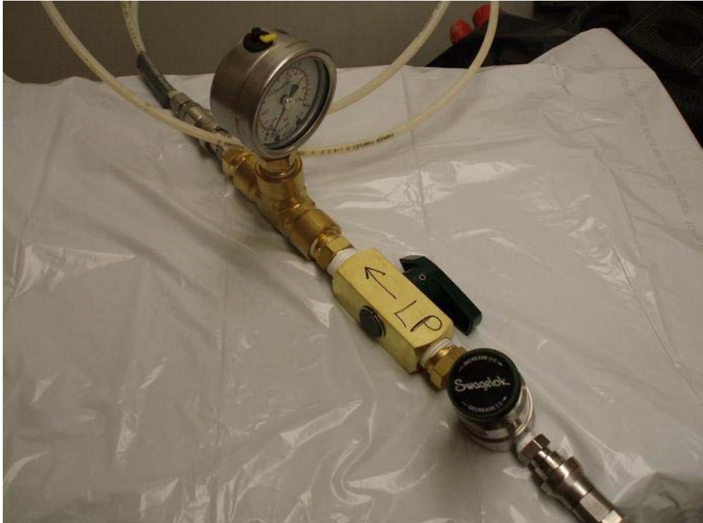
Figure 5. Low Pressure Regulator control, marked Swagelok®, is closed when turned fully counter-clockwise. Regulator has a maximum input pressure of 1000 psi and maximum output of 10 psi. Plug valve is open.
