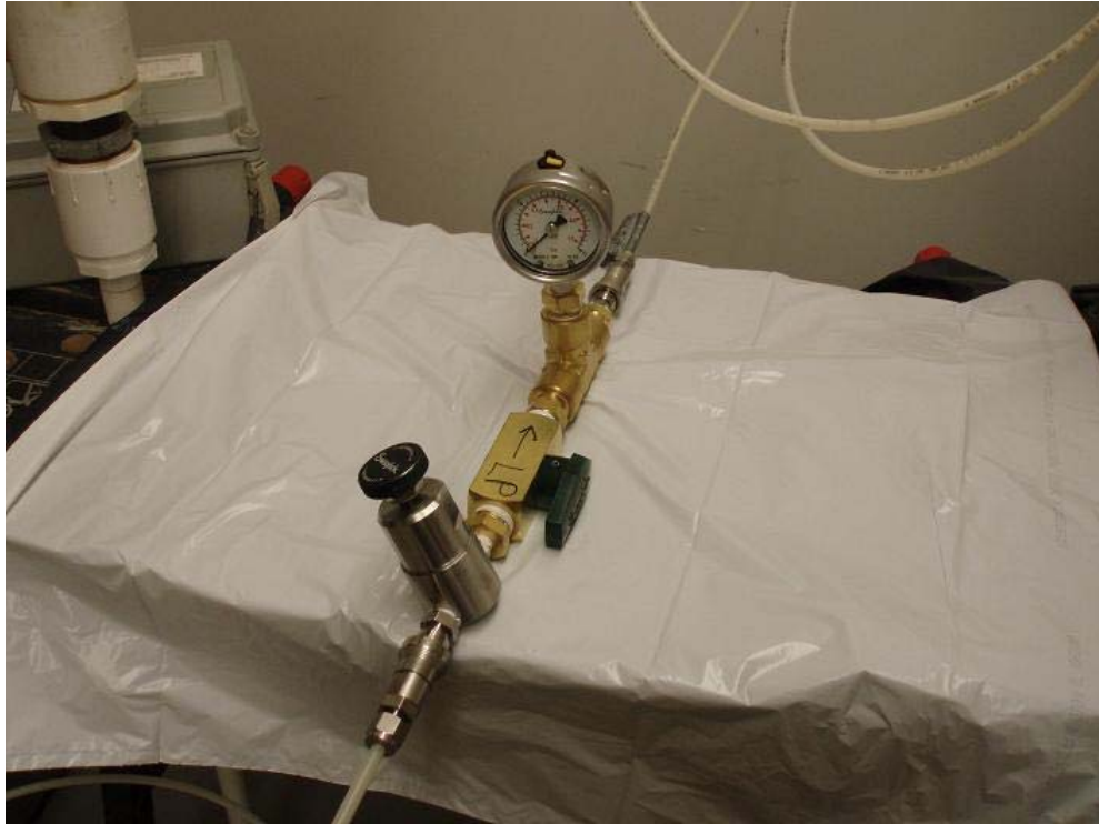
Figure 2. Low Pressure Regulator Manifold consisting of three components from bottom of picture; low pressure gas regulator, plug valve, and pressure gauge.
