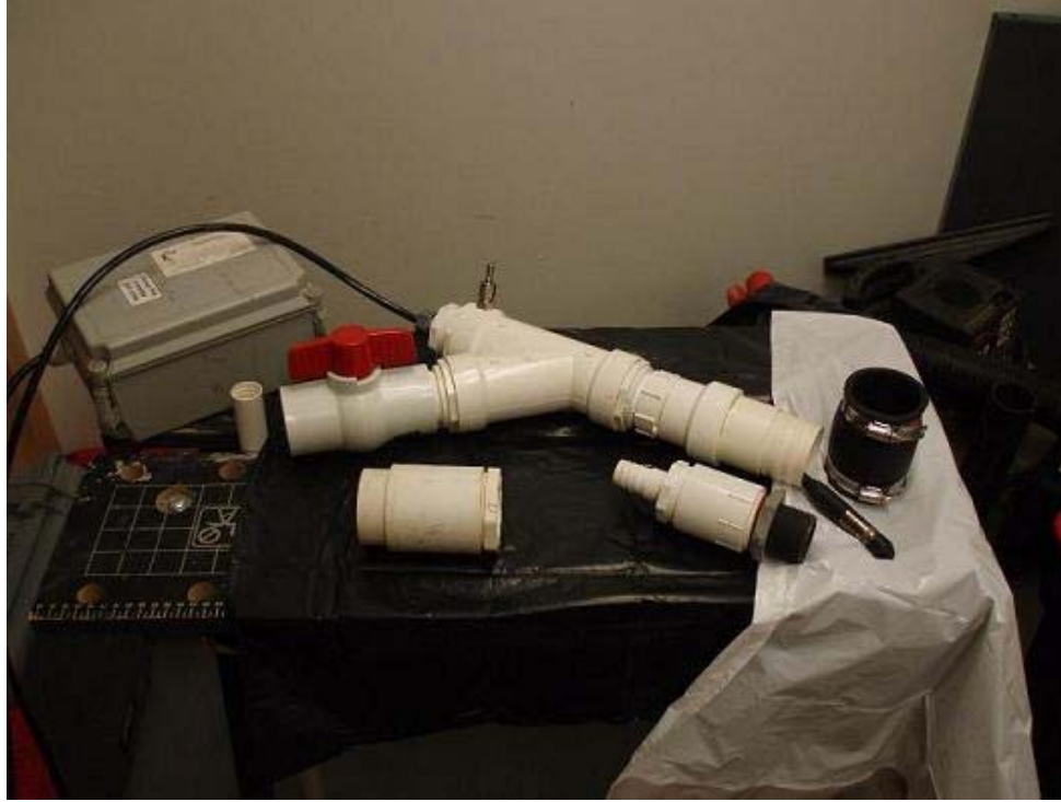
Figure 1. Well Head Manifold with transducer installed and several well pipe adapters. The Telog® data logger is the gray box on the left.
