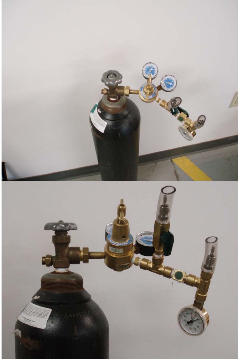
Figure 3. Two views of the Nitrogen tank with tank regulator installed. Upper view shows two gauges on the regulator. The one closest to the tank (HP gauge) indicates tank pressure. The other (LP gauge) indicates the pressure on the output of the regulator. The third gauge seen in the both photos at the lower right also indicates regulator output pressure but with a more precise scale than the LP gauge. In the lower photo is a view of two quick-connect
