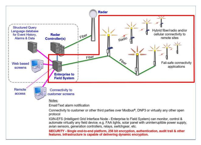
Figure 7. DigitaLogic IGIN-EFS Obstruction Lighting Control System [3]
