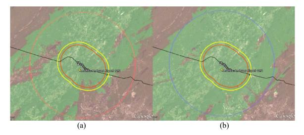
Figure 19. The 500-ft AGL Viewsheds: Radars HSR-01 (a) and HSR-02 (b)
