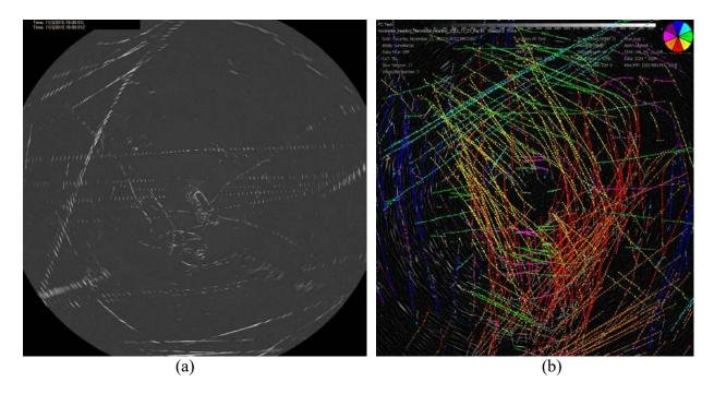
Figure 5. Unprocessed Radar Image (a) and Radar Image Processed by HARRIER Server (b) [5]
