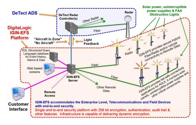
Figure 2. HARRIER ADLS Connected to Other ADLS Components [3]
