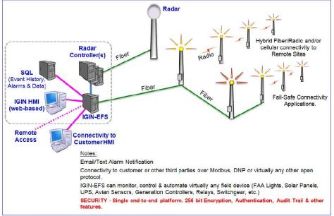
Figure 1: IGIN-EFS example showing typical ADLS components
