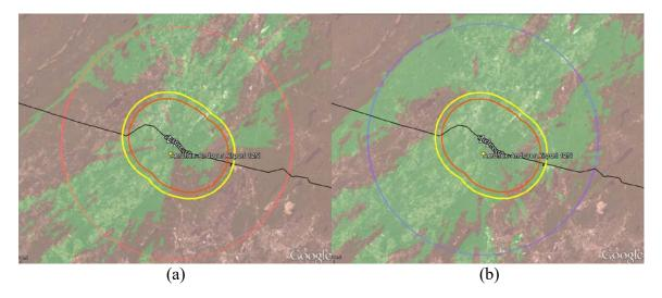
Figure 18. The 250-ft AGL Viewsheds: Radars HSR-01 (a) and HSR-02 (b)
