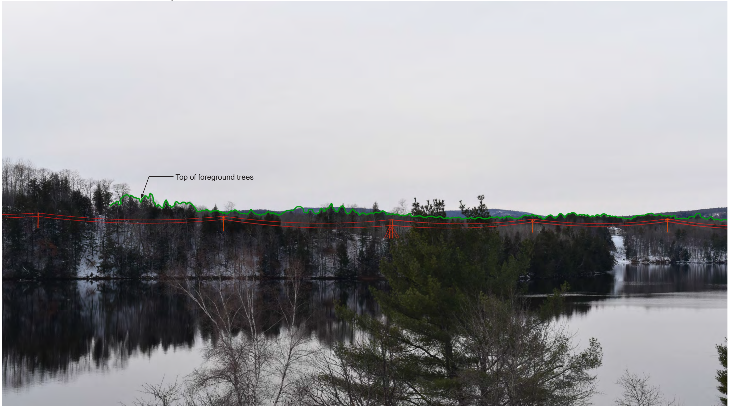
Viewpoint 7 (model overlay) - View looking west from the Route 201 Overlook in Solon toward the Project. No project visibility looking in this direction. Red lines represent conductors that are located behind the existing vegetation.
