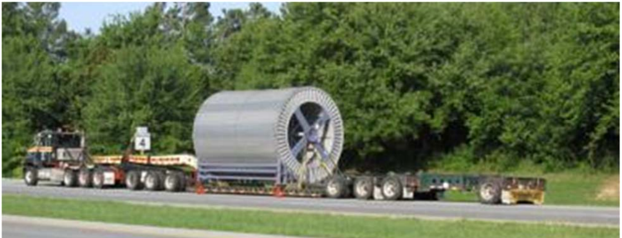
Figure 10- Oversized Reel Transport, 4,724 feet of 230kV Cable
