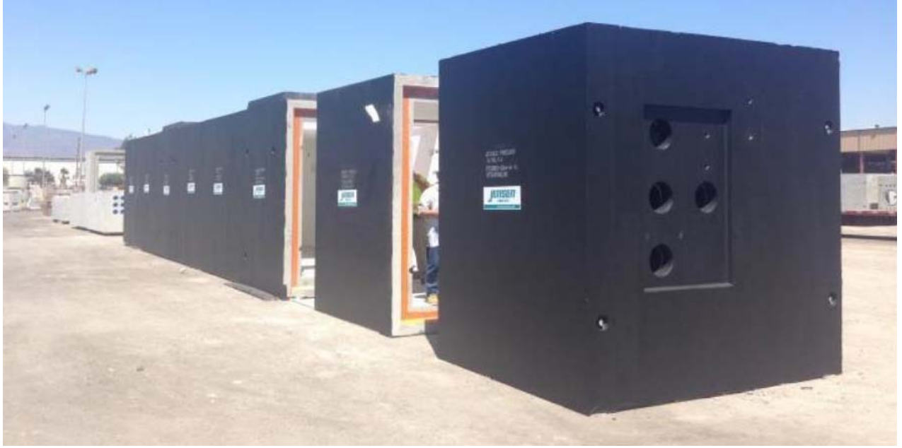
Figure 3 - 500kV Splicing Vault
