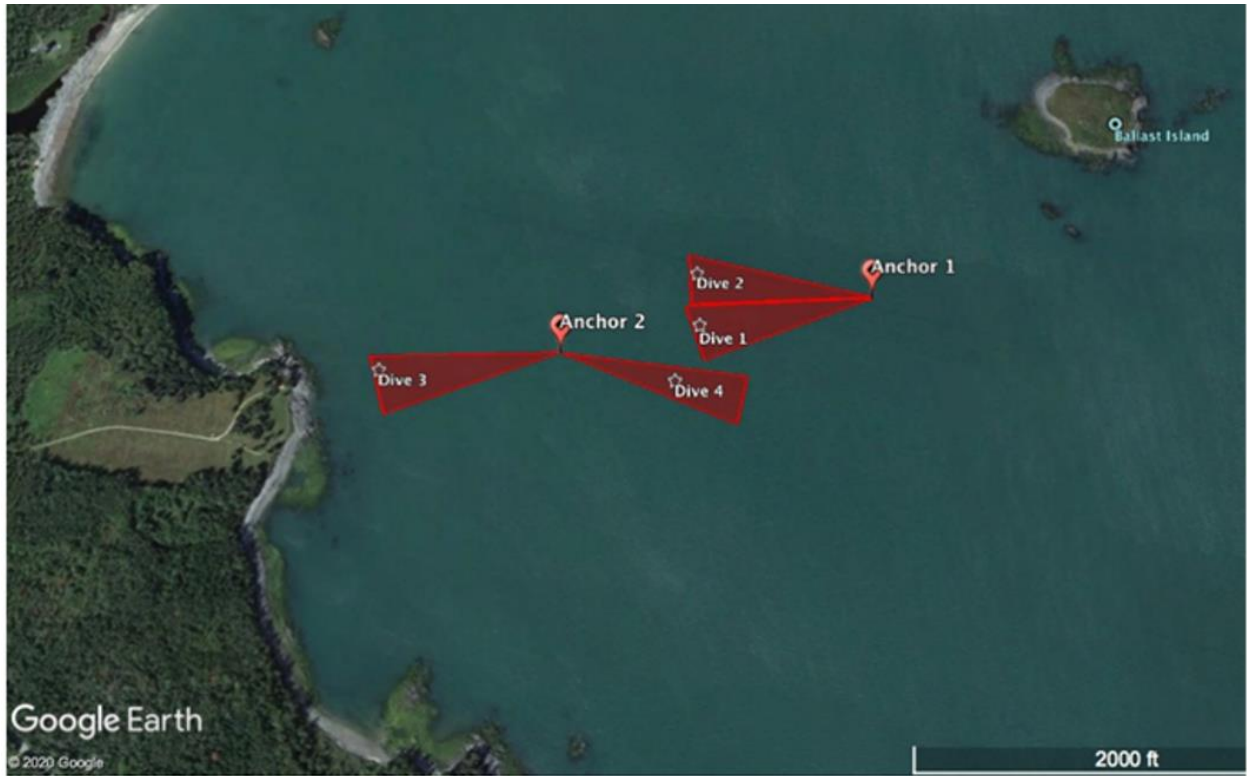
Figure 1: Dive area covered based on average heading and maximum tether length.
