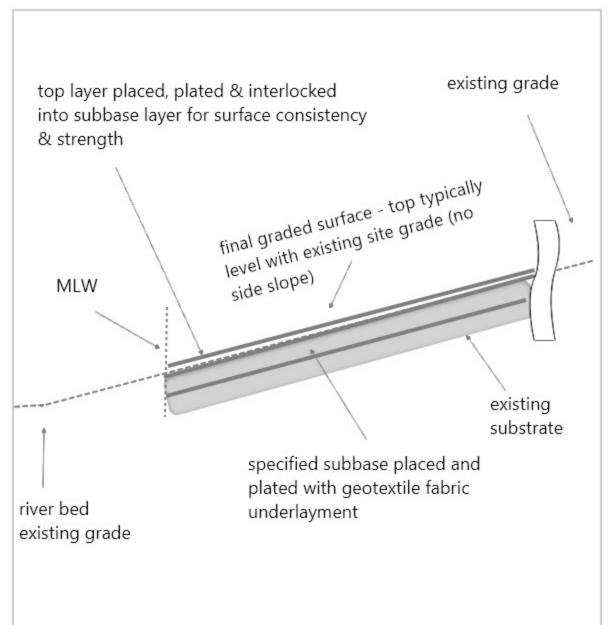
Note: estimated depth of stone top & sublayer 12" or less in lower sections as necessary for stability not to exceed volume as specified
