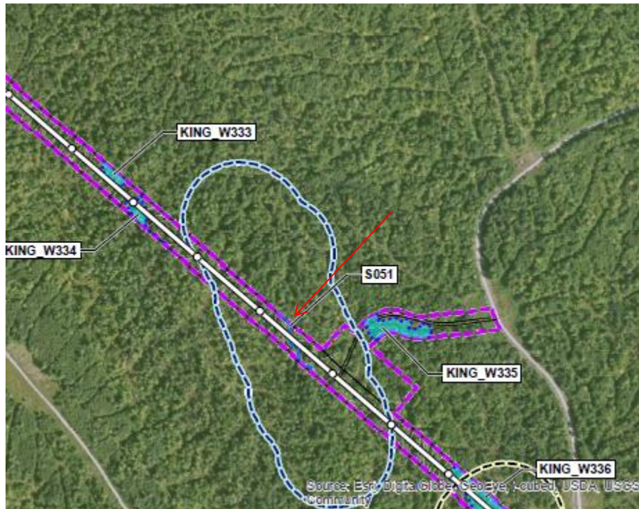
Proposed generator lead crossing of stream S051. From Figure 22 Delineated Natural Resource Map by Stantec Consulting.
