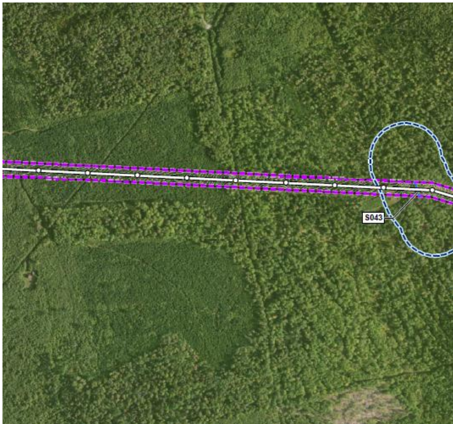
Proposed generator lead crossing of stream S043. From Figure 19, Delineated Natural Resource Map by Stantec Consulting.
