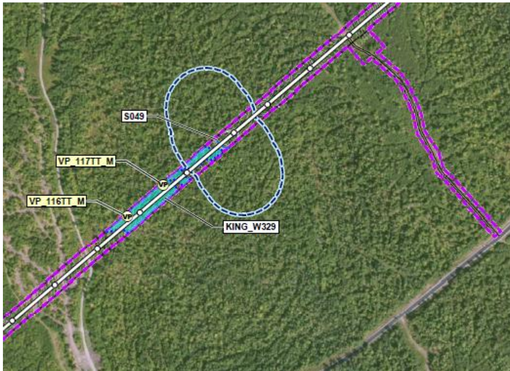
Proposed generator lead crossing of stream S049. From Figure 21 Delineated Natural Resource Map by Stantec Consulting.
