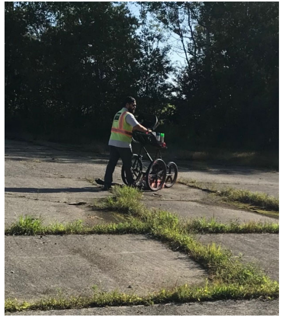
GPRS performing grid pattern scanning with utility cart GPR
