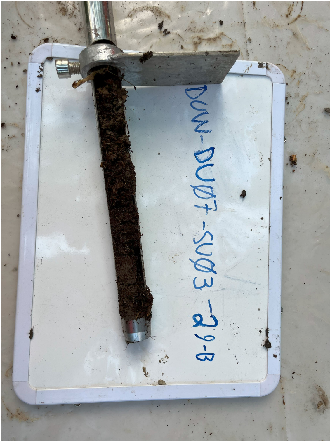
PHOTO 001: Photograph of core with highest PID reading within DU07-SU03. Peak PID reading measured at 6" below ground surface (bgs)
