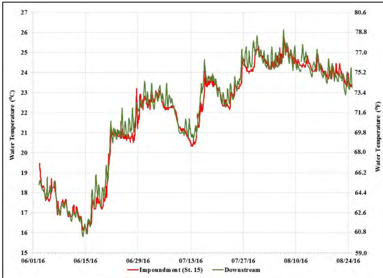
Figure 4-9 Hourly Water Temperature at the Lake Trophic Sample Site in the Impoundment (Station 15) and at the Riverine Sample Site Downstream of the Shawmut Dam
