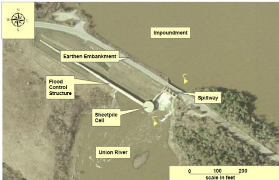
Figure 2. Graham Lake Development facilities (Source: U.S. Geological Survey, 2013, as modified by staff).
