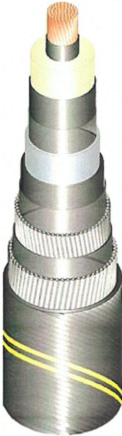
Photo 2 -- HVDC Light cables are lightweight and oil-free. In operation, they have a neutral electro-magnetic field. (photo courtesy of ABB)
