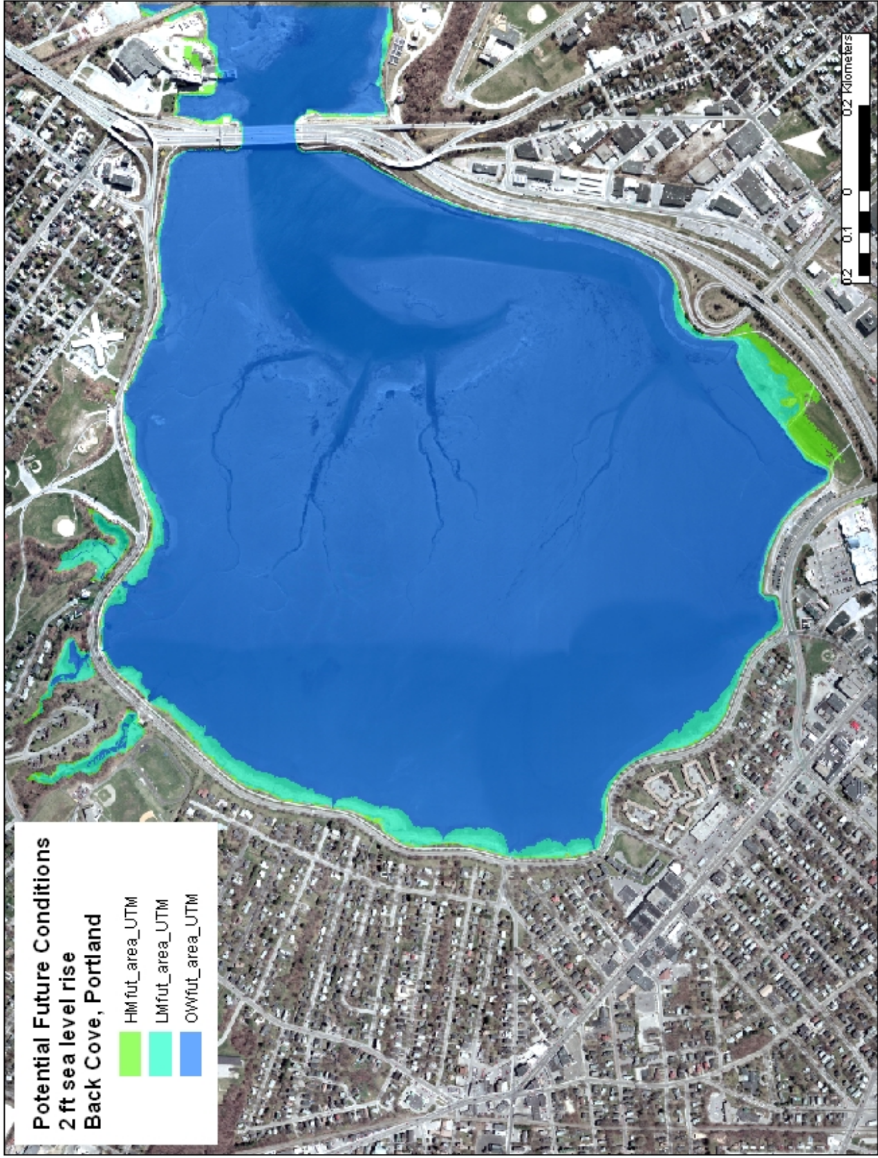
Figure 24. Simulation of potential future marsh conditions at Back Cove after 2 feet of sea level rise. Note what little high marsh existed is pinched out by transgressing low marsh. The existing soccer field (southeast) appears to be the only area where the high marsh may have room to transgress, along with smaller finger marshes at the northern side.
