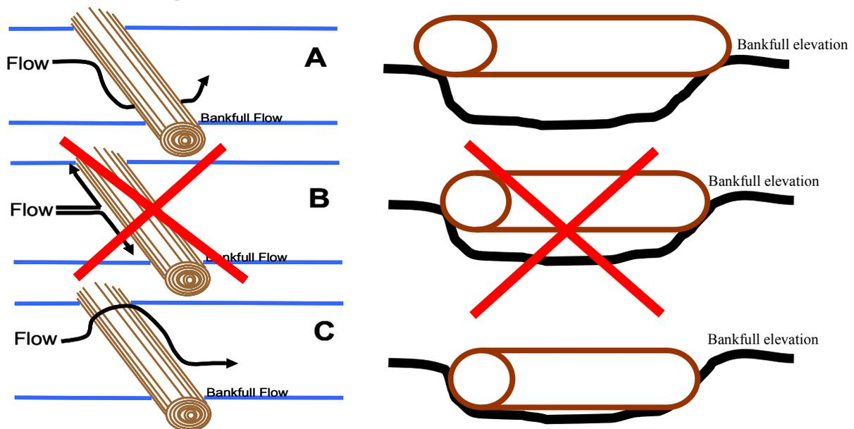
**Figure 2.** A) adding smaller wood on each side of the stream to concentrate flow over or under the large wood and protect banks from dispersal flow. B) over time a pool will likely form with the material moving down stream to form a pool tail/riffle habitat complex. Note this type of treatment is specifically for a stream identified by DIFW or DMR as having an over widened channel.
