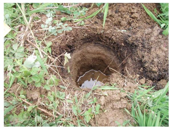
Photograph Five. TP 5B – Tunbridge "like" soils after a rain with bedrock @ 18". 06/19/09.
