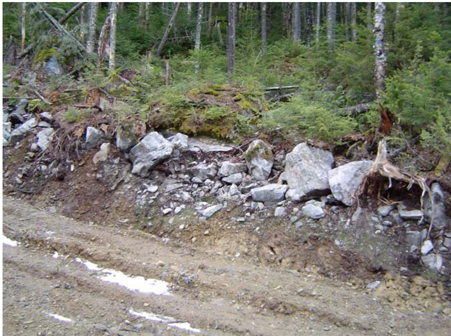
Photo 3: Existing road profile at Seven Ponds TWP at 2,500' +/-. Photo illustrates stony surface horizon over deep glacial till substratum. Photographer A.F. 11/12/2003.
