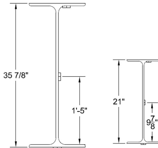
Figure 3 - Gage location on Indian Purchase cross section of floor beams and stringers respectively
