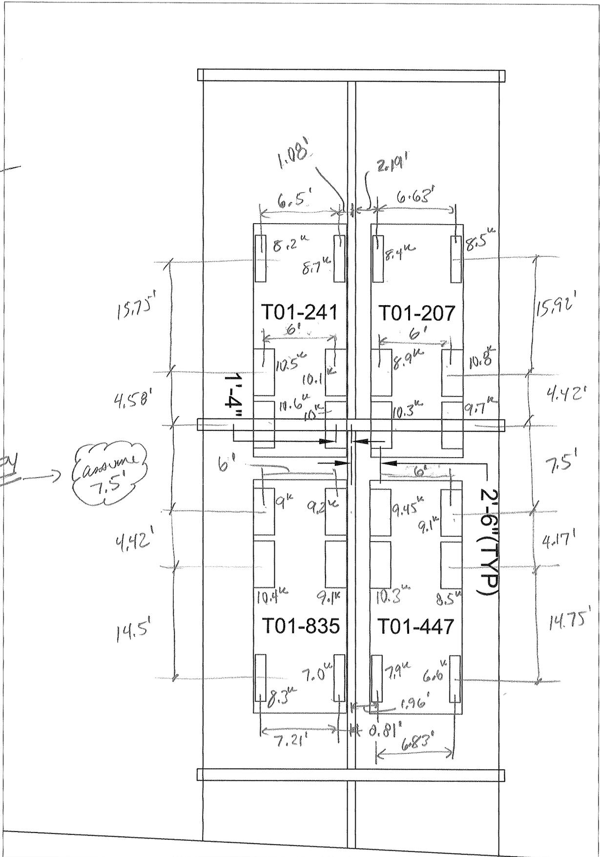
Trucks traveled from end of span to past midspan during test
