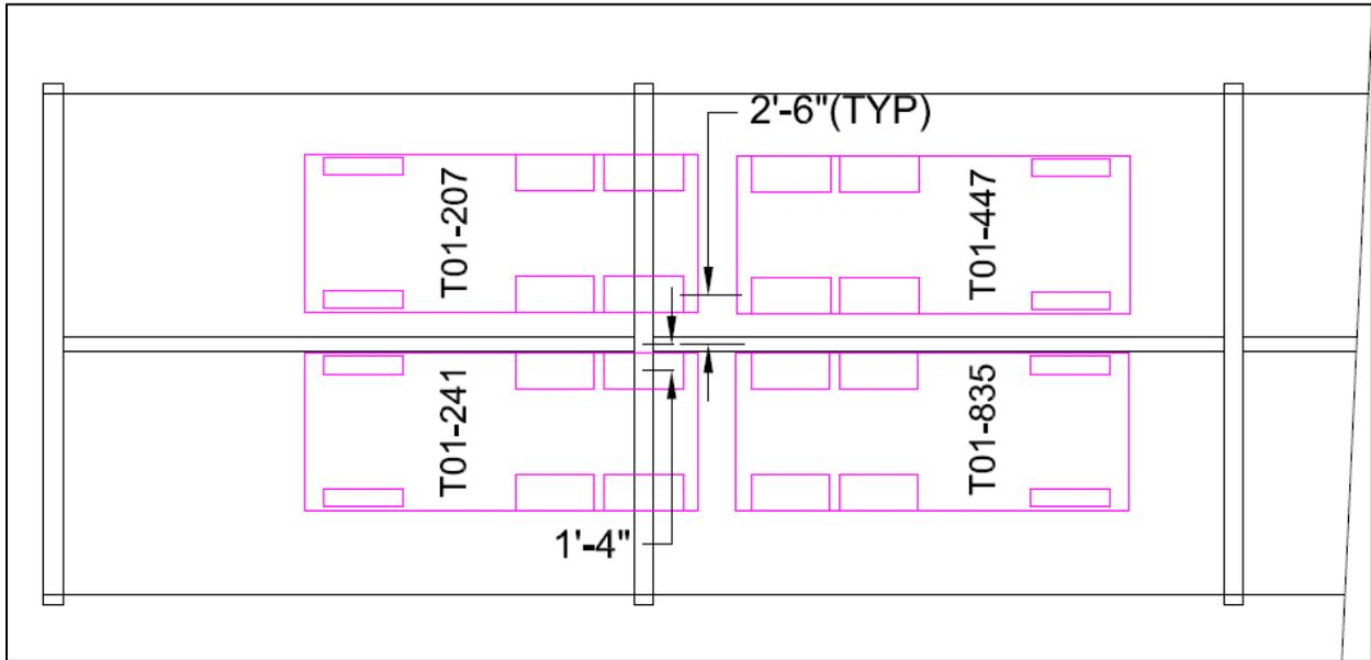
Figure 10 – Four truck loading of Brownville
