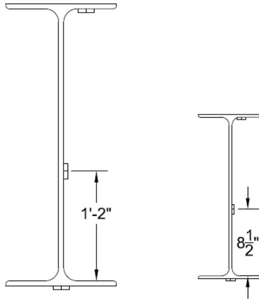
Figure 2 - Gage location on Chester cross section of floor beams and stringers respectively
