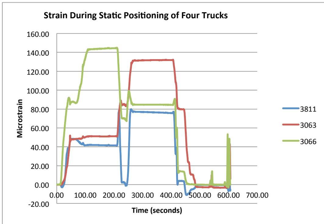
Figure 18 – Plot of peak strain during static positioning of four trucks across two floor beams for Brownville (No. 3222)
