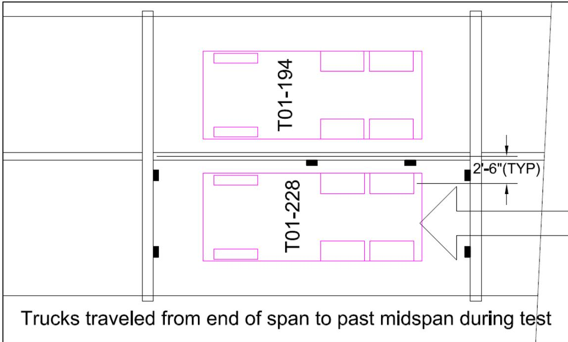
Figure 12 – Two truck loading of Chester
