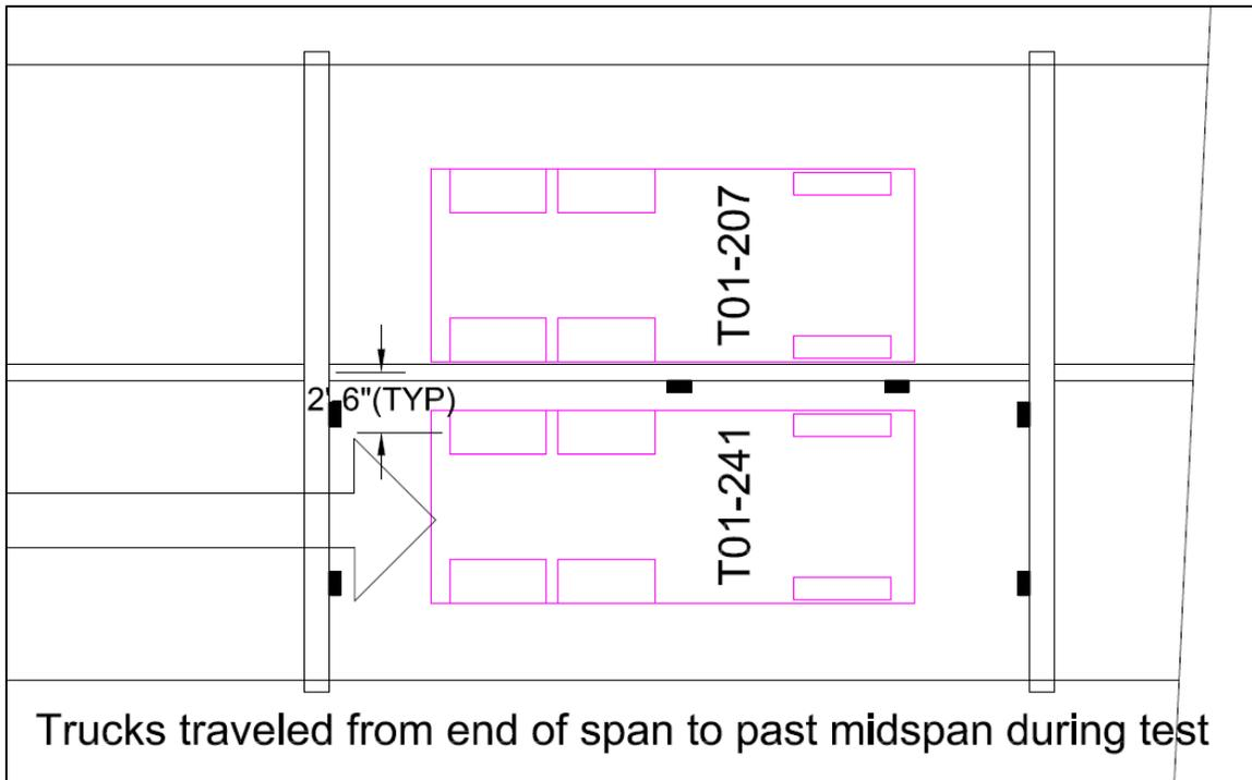
Figure 9 – Two truck loading of Brownville
