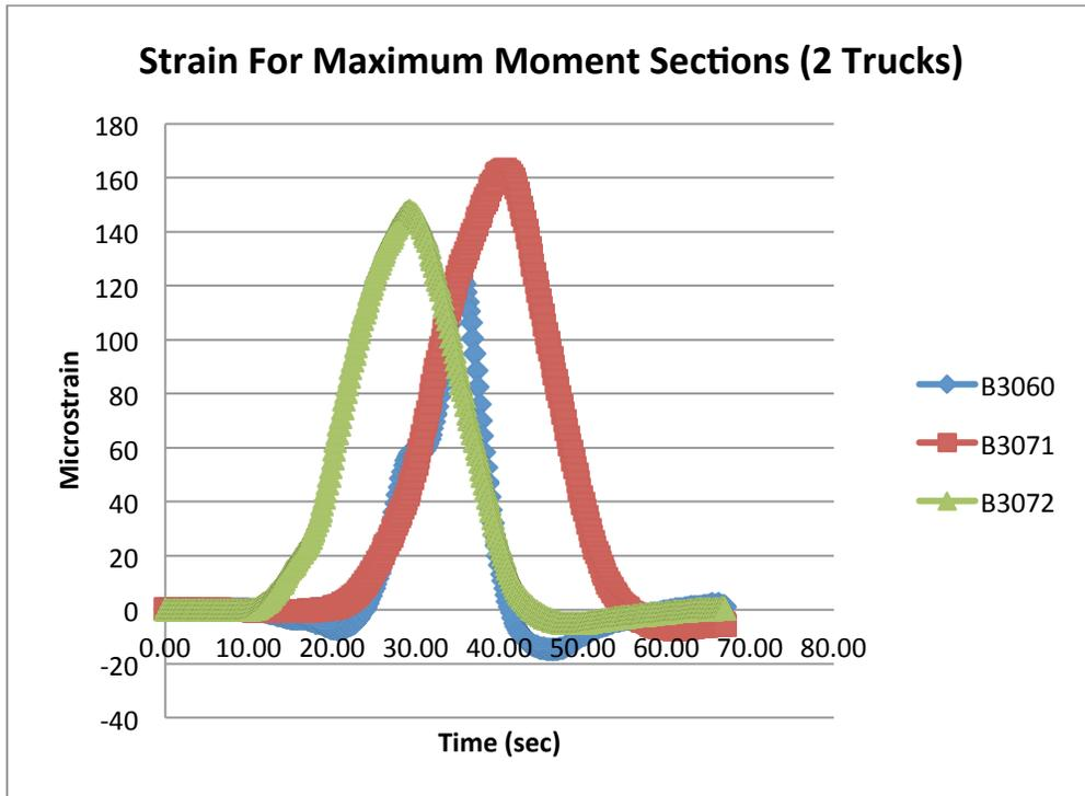
Figure 19 – Chart of strain during 2 truck load case for Indian Purchase (No. 3666)
