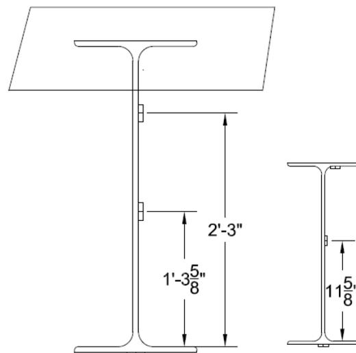
Figure 1 - Gage location on Brownville cross section of floor beams and stringers respectively
