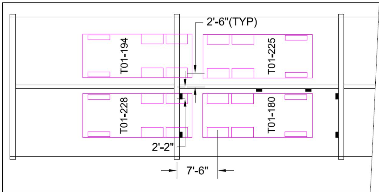
Figure 13 – Four truck loading of Chester
