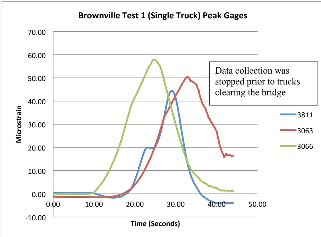
Figure 17 – Plot of strain during first test at Brownville (Bridge No. 3222)
