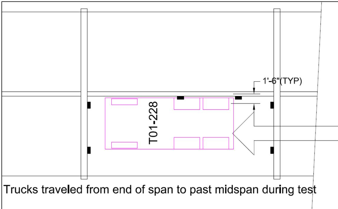
Figure 11- One truck loading of Chester
